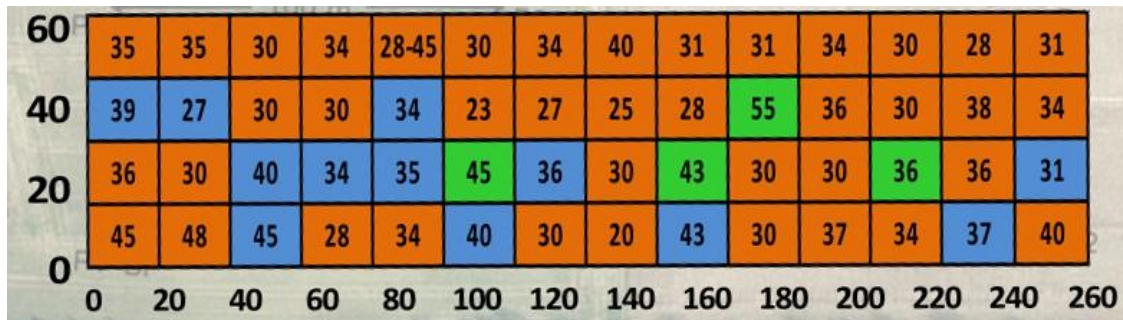
Fig. 7: Borders between A and B horizons in the field [cm]. Colours depict the soil type: orange: Luvisols, blue: stagnic Luvisols, green: Cambisols. Soil assessment was done by the group of K. Totsche (Univ. Jena) within the Research Units program.
