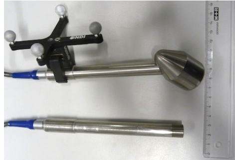
Figure 6.1.: Gamma probes. Top: high-energy (511 keV ) gamma probe. Bottom: 140 keV gamma probe.
