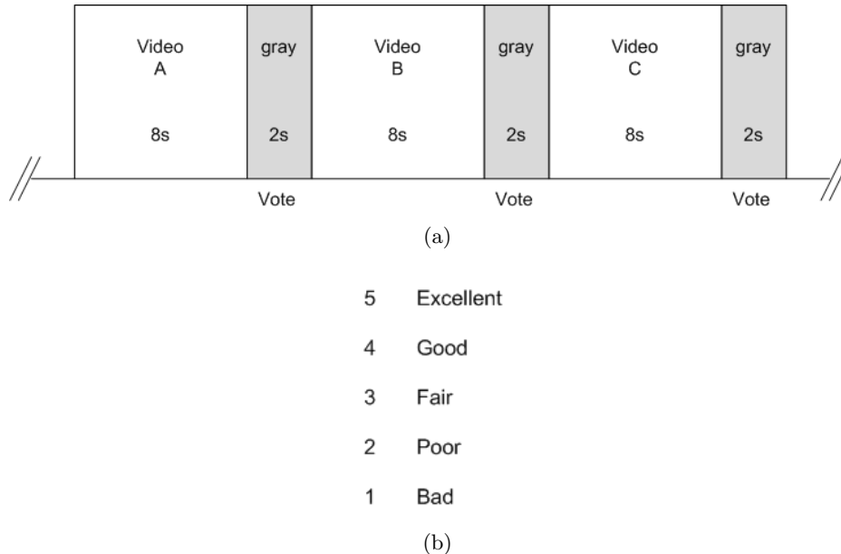
Figure 2.2: Absolute Category Rating (ACR) [ITU99]: (a) Presentation structure; (b) rating scale.
