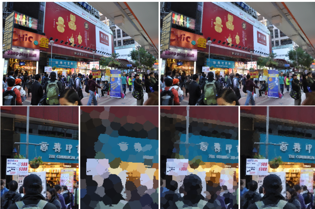
Figure 2.4: Top row: Original image and SLIC superpixels [5] with 8000 superpixels. Bottom row: Close up with 2000, 8000 and 32000 superpixels.
