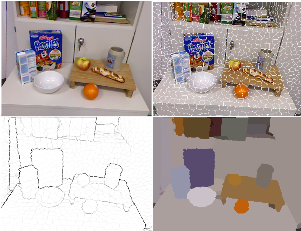
Figure 4.1: Top: Input RGB-D image (only colour is shown) and depth-adaptive superpixels. Bottom: Ultrametric contour graph indicating boundary strength and final segments.
