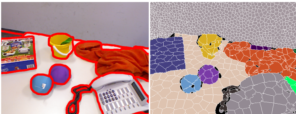
Figure 4.2: Left: Colour image of a possible manual ground truth annotation. Right: s-DASP image segmentation (colours) using depth-adaptive superpixels (white lines).
