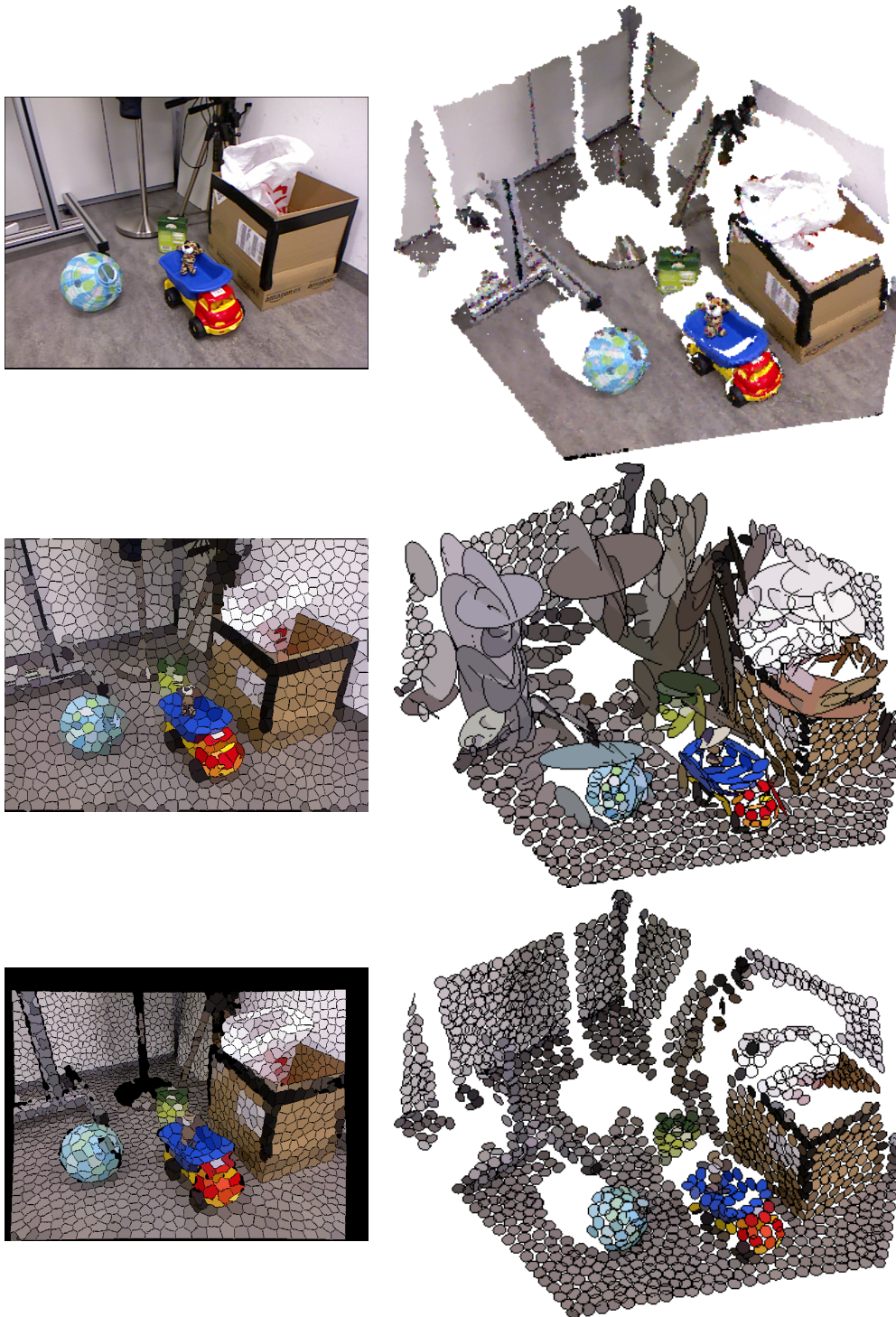
Figure 3.3: Top: Original colour image and corresponding 3D point cloud. Middle: ASP/SLIC superpixels with constant density and corresponding 3D superpoints computed from point positions. Bottom: DASP superpixels with depth-adaptive density and corresponding 3D superpoints. Black pixels at the border and at some object edges indicate missing depth data.
