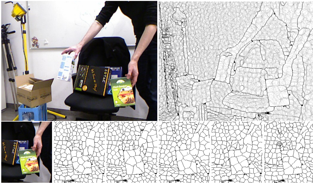
Figure 5.4: Top left: Colour part of the RGB-D input image. Top right: Mean image of border images for 12 possible DASP superpixel oversegmentations. Bottom: Detail of the full colour image and a set of different but equally likely DASP oversegmentations.
