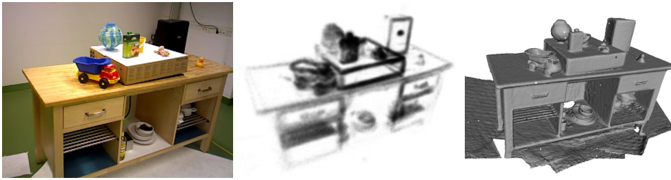
Figure 8.2: Comparison of sparse event-based map (middle) against a mesh created by the dense mapping algorithm KinectFusion (right). The color image (left) is provided for reference.
