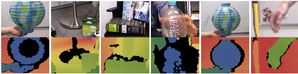
Figure 3.5: From left to right: A selection of unfavourable conditions under which the PrimeSense sensor fails to measure depth values: too close, too shiny, too steep, transparency, missing depth information due to the sensor baseline and a non-constant time-offset between colour and depth frames noticeable for fast motions.
