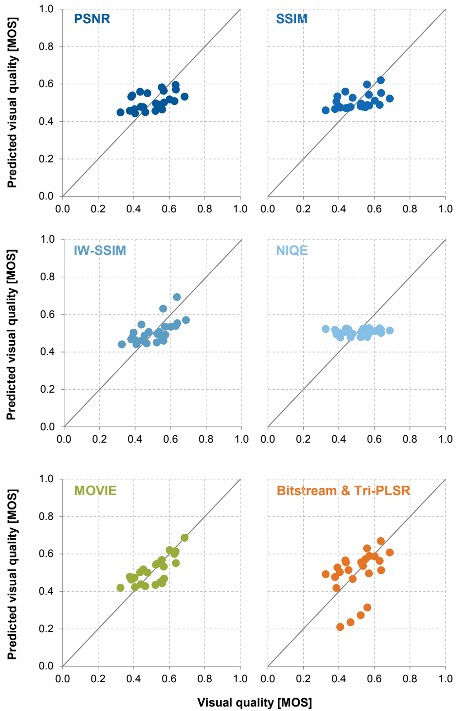
Figure B.19.: Scatter plots of the prediction results of the bitstream-based example metric built with trilinear PLSR (Tri-PLSR) compared to PSNR, SSIM, IW-SSIM, NIQE and MOVIE for the LIVE data set, showing the visual quality y against the predicted visual quality \hat{y}
