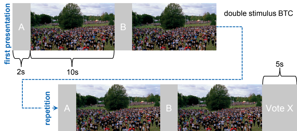
Figure 2.7.: Double stimulus BTC: presentation of reference A and test condition B , repeated once and then followed by a voting block
