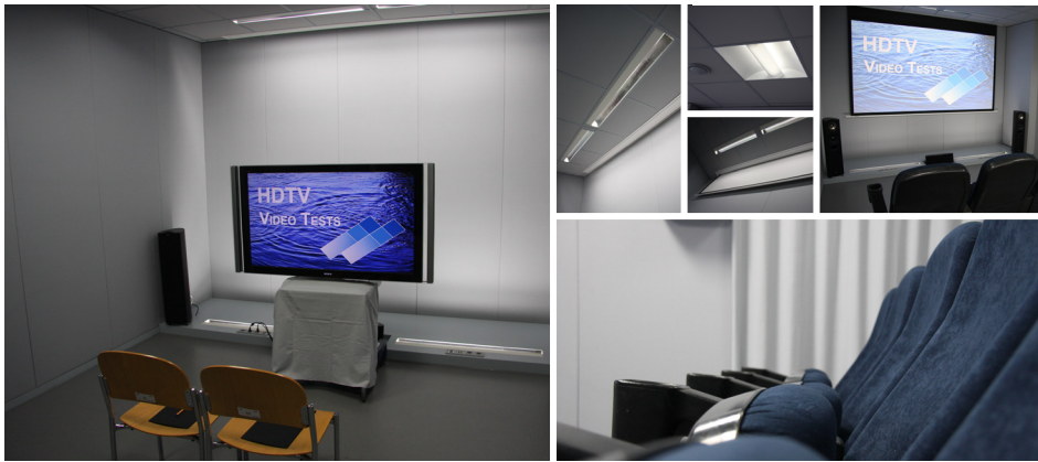
Figure 2.3.: ITU-R BT.500 compliant subjective testing laboratory at TUM: controlled lighting, colour-neutral mid-grey background, adaptability to different displays and test setups
