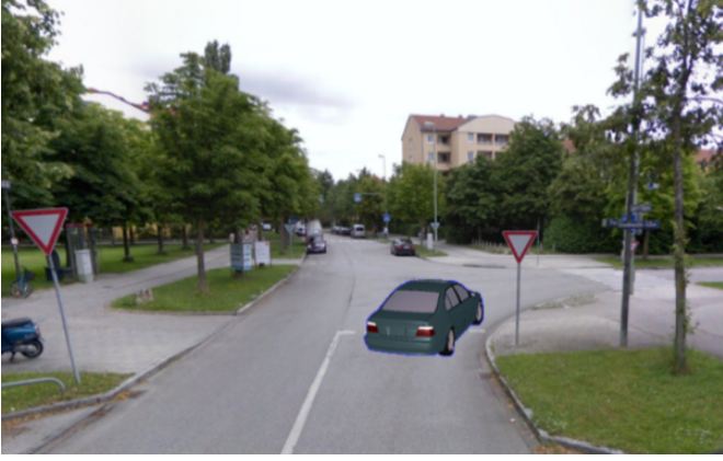
Figure 3: The predicted vehicle position is drawn onto the received camera image.
