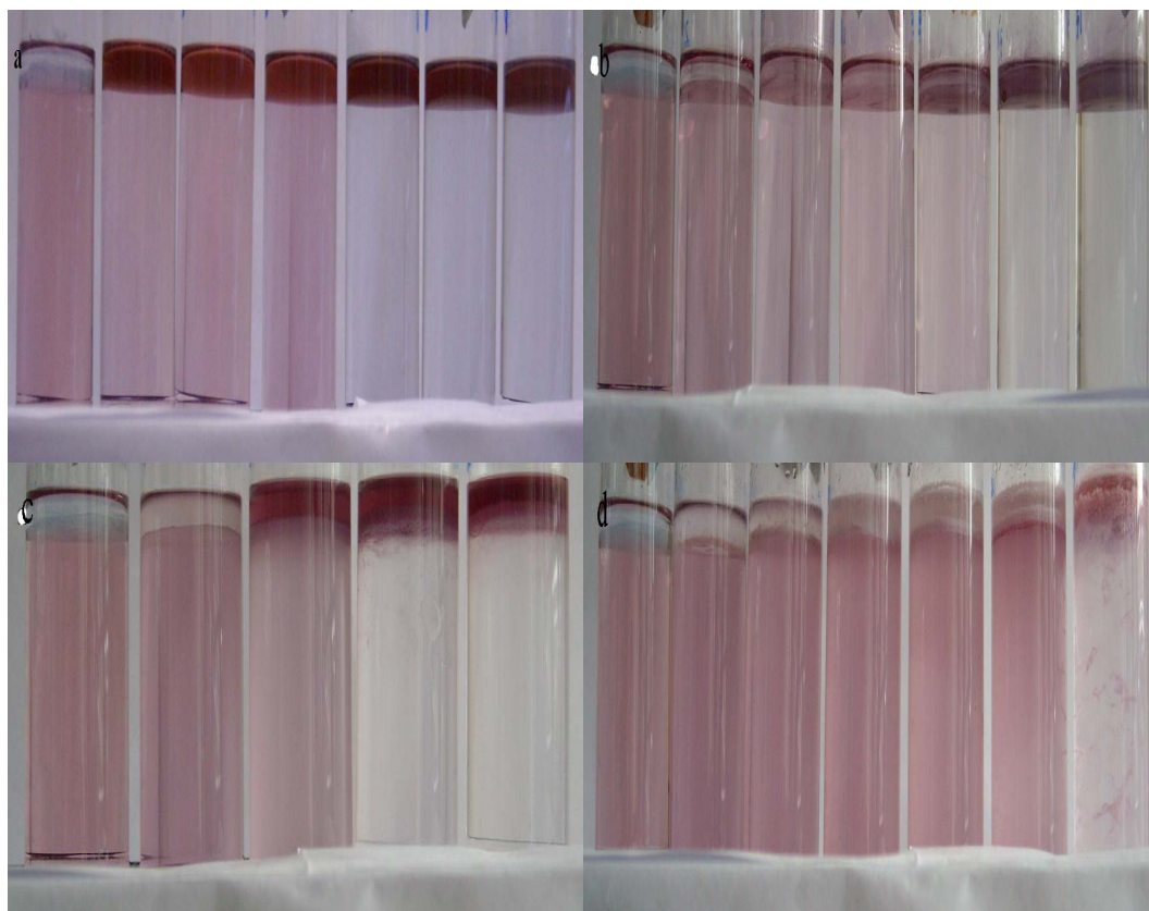
Figure 3. Photos for extraction of Au-NPs (0.05 mmol/L) from water to n-hexane using different concentrations of ligand. a) DDT. b) ODT. c) DDA. d) ODA
