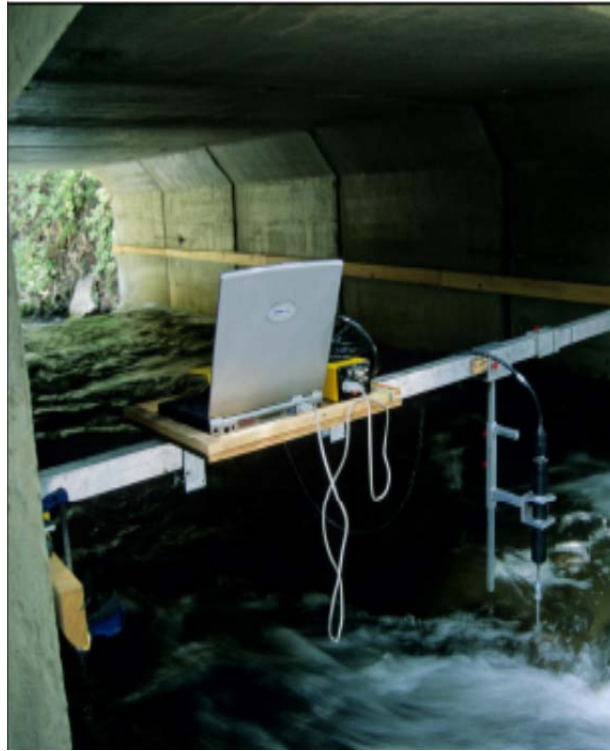
Figure A3: Typical measurement of the upstream and Downstream Velocity (after Blank, 2008).
