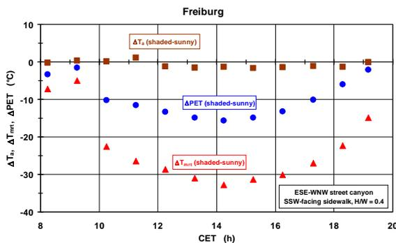
Figure 2: 1h mean values of the differences  $\Delta$  of  $T_a$ ,  $T_{mrt}$  and  $\Delta PET$  between a shaded (by tree canopies) and sunny SSW-facing sidewalk of an ESE-WNW street canyon ( $H/W=0.4$ ) in Freiburg on a typical Central European summer day (July 24, 2008).
