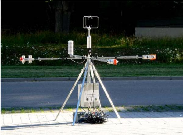
Figure 1: Human-biometeorological measuring station used in investigations on thermal comfort in Freiburg [5-8].
