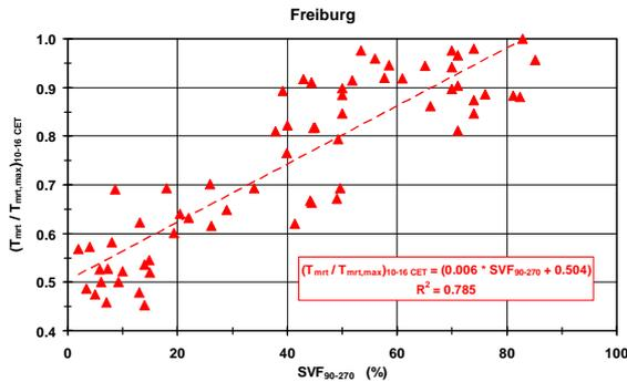
Figure 4: Relationship between mean values (10-16 CET) of  $T_{mrt}/T_{mrt,max}$  ( $T_{mrt,max} = 64.1$  °C) and  $SVF_{90-270}$ , based on experiments at different sites in Freiburg on typical summer days 2007-2010.
