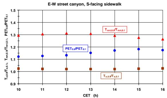
Figure 6: Simulated ratios of  $T_a$ ,  $T_{mrt}$  and PET between the albedo values  $a=0.9$  and  $a=0.1$  of the building walls of an E-W street canyon ( $H/W=1$ ), related to the S-facing sidewalk (width: 1 m).
