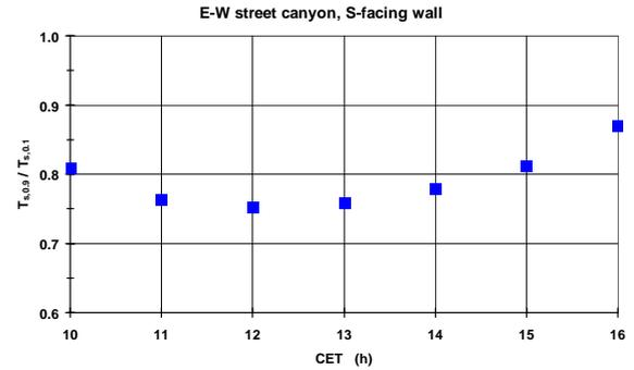
Figure 5: Simulated ratio of the surface temperature  $T_s$  between  $a=0.9$  and  $a=0.1$  of a S-facing wall of an E-W street canyon ( $H/W=1$ ) for a heat wave day in August 2003,  $a$ : albedo.
