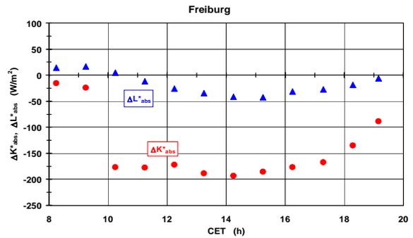
Figure 3: 1h mean values of the differences  $\Delta$  of the sums  $K^*_{abs}$  and  $L^*_{abs}$  of the short- and long-wave radiant flux densities from the three-dimensional environment absorbed by the human-biometeorological reference person between a shaded (by tree canopies) and sunny SSW-facing sidewalk of an ESE-WNW street canyon ( $H/W=0.4$ ) in Freiburg on a typical Central European summer day (July 24, 2008).
