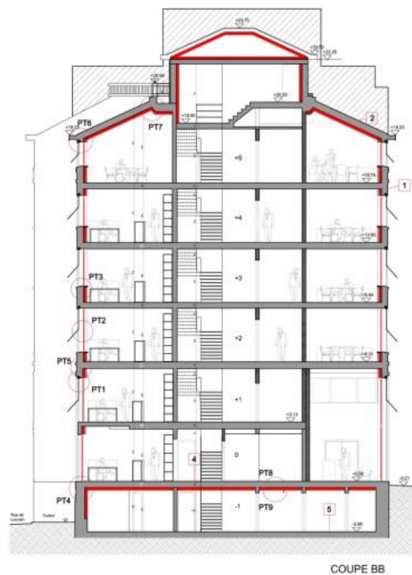
Figure 1: Study with location of the thermal bridges in the building section.
