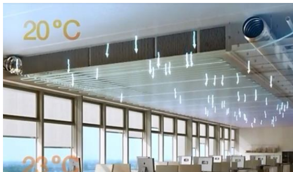
Figure 8: Cooling from the ceiling system (Interalu) and the use of thermal mass.
