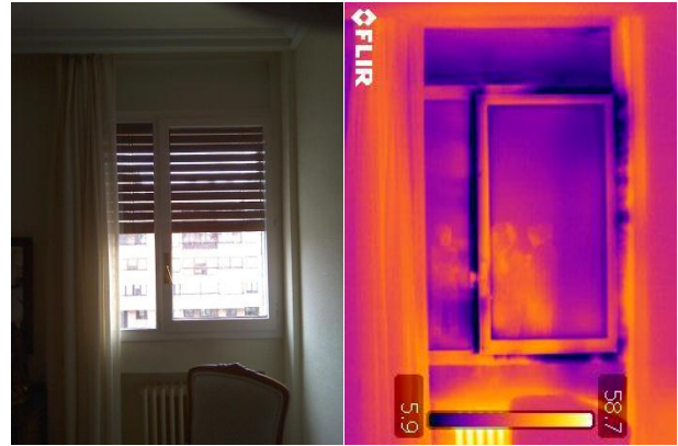
Figure 5: Photography and thermography of one window during the blower door test under depression.
