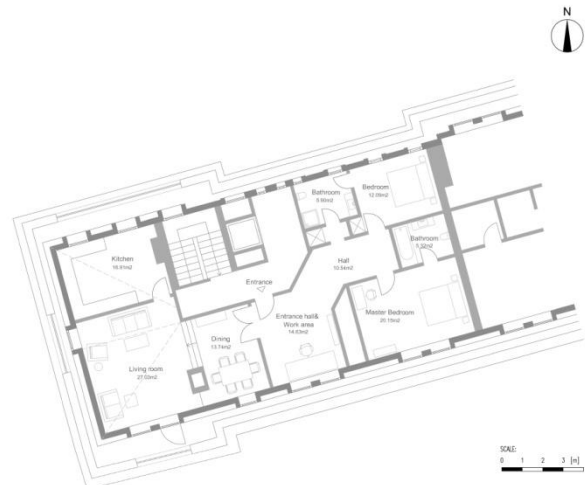
Figure 3: Plan of Flat 30 in Royal Standard House (redrawn by the author, based on the information from the Nottingham City Council planning department [11] and current flat layout).
