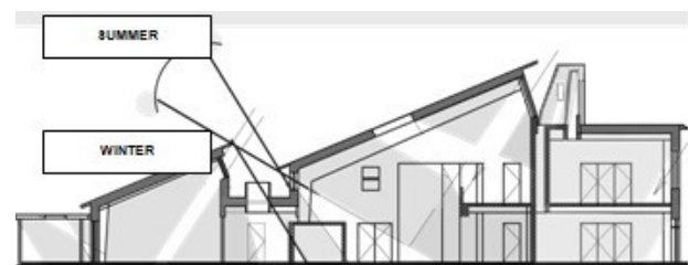
Figure 4: Section of St-Lukes C&E Primary School showing the daylight strategies (source from Architype and redrawn by the author)
