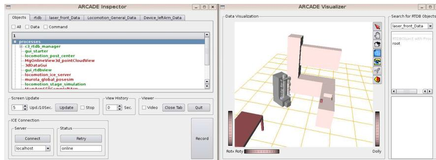
**Fig. 3** The *ARCADE Inspector* lists the tree of all database objects, provides access to the object data and a record functionality. The *ARCADE Visualizer* provides a 3D visualization of the current system state.
