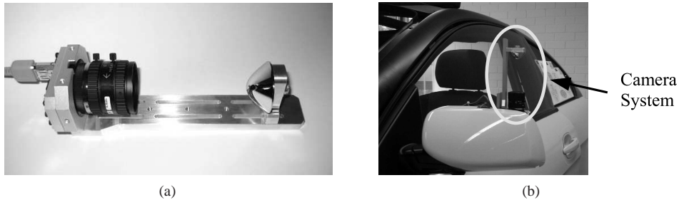
Fig. 2: The omnidirectional camera system (a): A perspective camera focuses on a hyperboloidal mirror and takes pictures with a field-of-view of 360^\circ . Our camera system integrated with the side-view mirror of a car (b).
