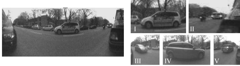
Fig. 3: Left: Panoramic image of the environment around a car door. Right: Different views and sizes of approaching and passing traffic participants due to the large field of view of the camera. The detection algorithm must be able to handle different sized objects (large (I) and very small objects (II)) and to robustly detect passing objects that differently appear in panoramic images (Different views of a passing car (front view (III), side view (IV) and rear view (V)).
