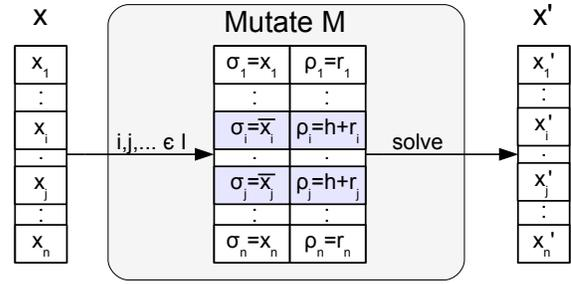
Fig. 4. Feasibility-preserving Mutate Operator. A certain amount of bits  $I$  are prioritized to flip. This set  $I$  deduced by the mutation rate.
