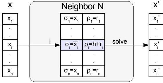
Fig. 3. Feasibility-preserving Neighbor Operator. One bit  $i$  is forced to flip with a high priority.
