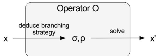
Fig. 2. PB solver based local search operator. Given is the solution  $x \in X_f$ . Following  $x$ , a branching strategy  $\rho, \sigma$  for a PB solver is deduced. With this branching strategy, the PB solver finds an feasible  $x' \in X_f$  automatically.
