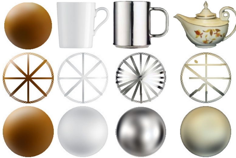
Figure 8.6: Estimated reflectance functions for several examples. Top : smoothed input images, Center : shading samples extracted by the user. Bottom : estimated reflectance function (even for tiny and textured objects), see Section 8.3.1 for details.
