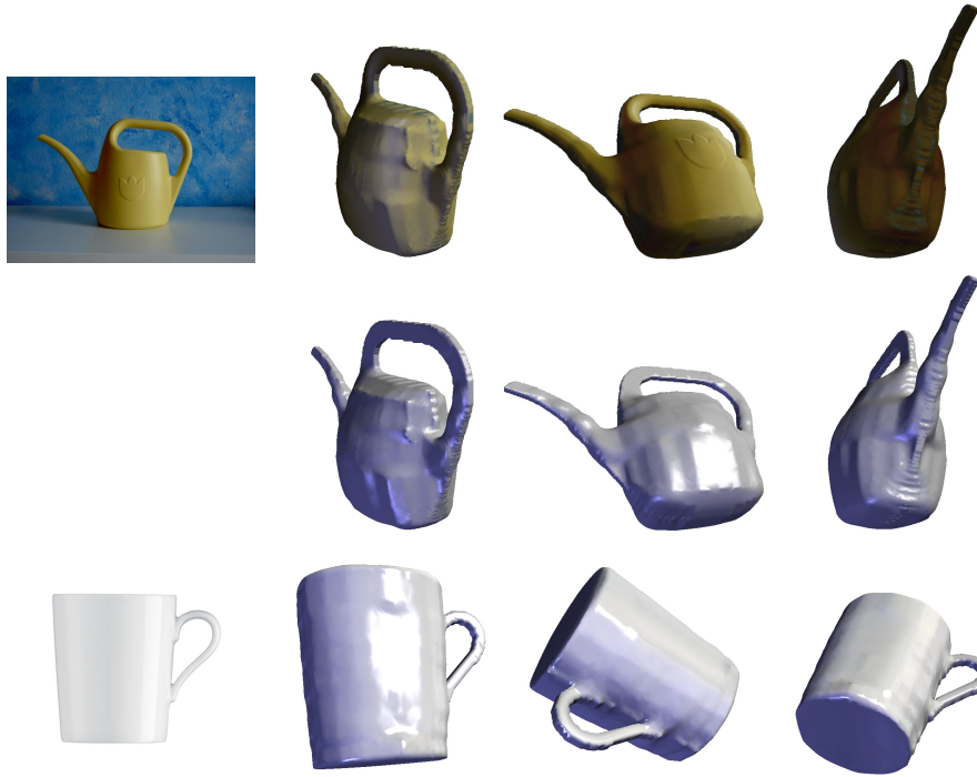
Figure 8.7: 3D reconstruction results with automatically estimated relative depth profile constraints based on shading information. The center row shows the reconstruction geometry without texture.
