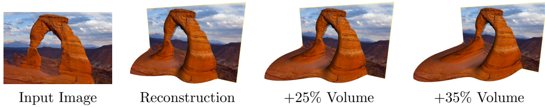
Figure 6.2: By interactively increasing the target volume, the reconstruction is intuitively inflated. Broader parts of the silhouette are inflated more than thinner ones.
