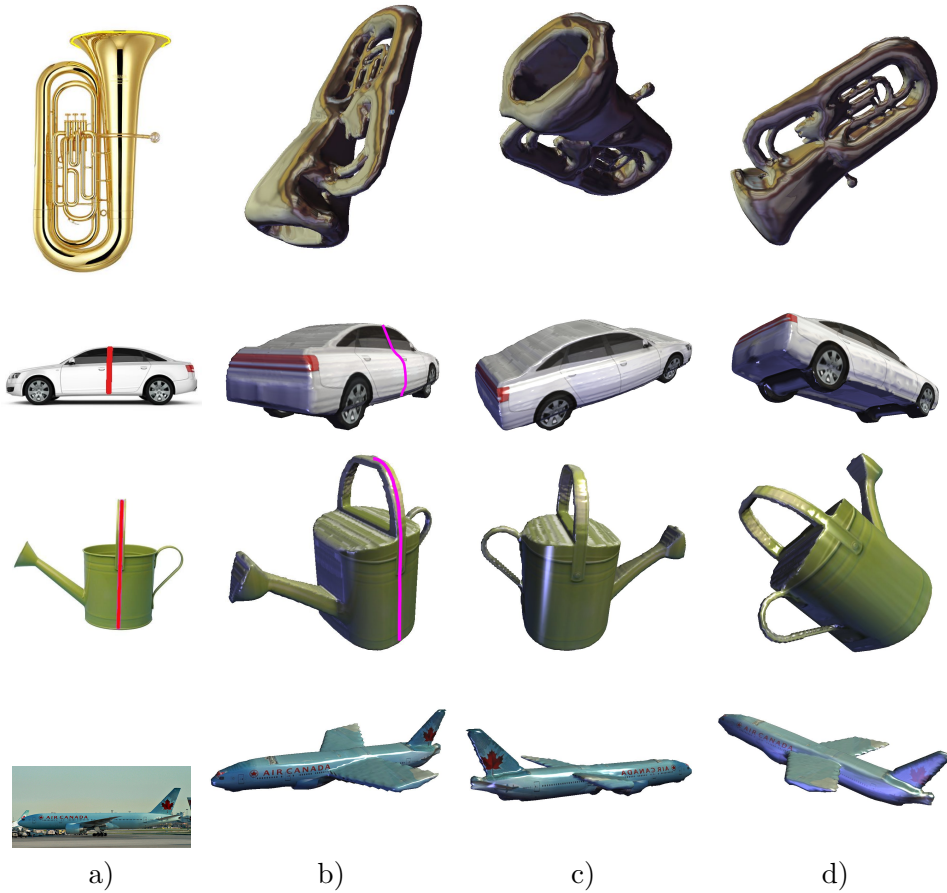
Figure 8.8: 3D reconstruction results with application of volume ratio constraints. a) Original images with relative depth profiles marked in red (location) and pink (depth function), b-d) Reconstructions with application of volume ratio constraints.
