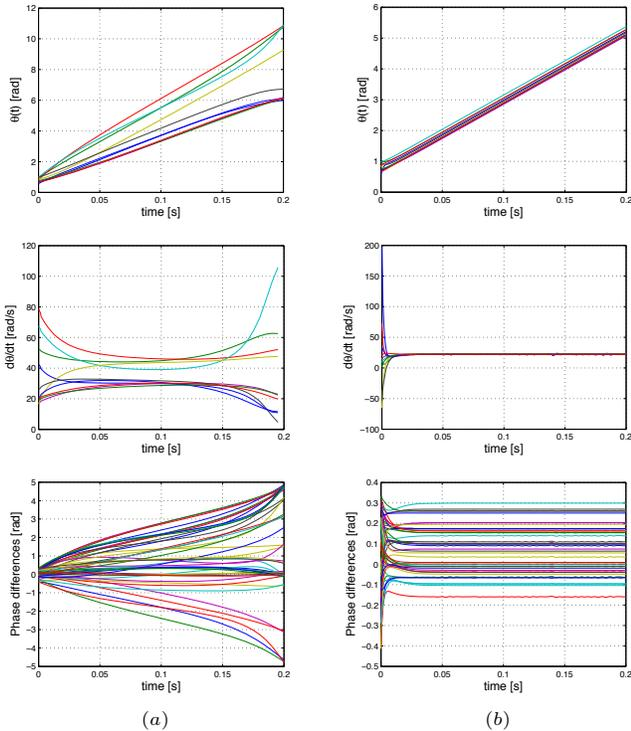
Fig. 2. Simulation results for a network of 10 oscillators, before (a) and after (b) applying controller
