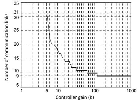
Fig. 3. Number of communication links needed to guarantee synchronization decreases as the controller gains increase
