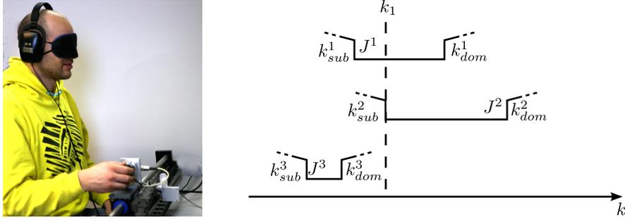
Fig. 1: A linear haptic interface (left) was used to determine the interval boundaries for  $k_1$ , which is identified using optimization techniques (right). Different cost functions  $J^{1\dots 3}$  are associated with individual participants.
