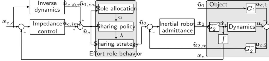
Figure 8: Overall scheme of the interaction control architecture embedding the effort-role behavior.
