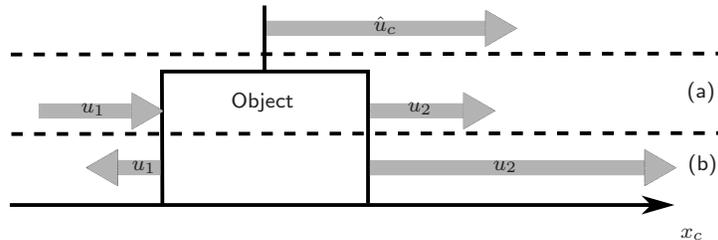
Figure 4: Illustrative example of input decomposition in a one-dimensional redundant task. (a) minimum-norm solution. (b) possible, but inefficient solution.
