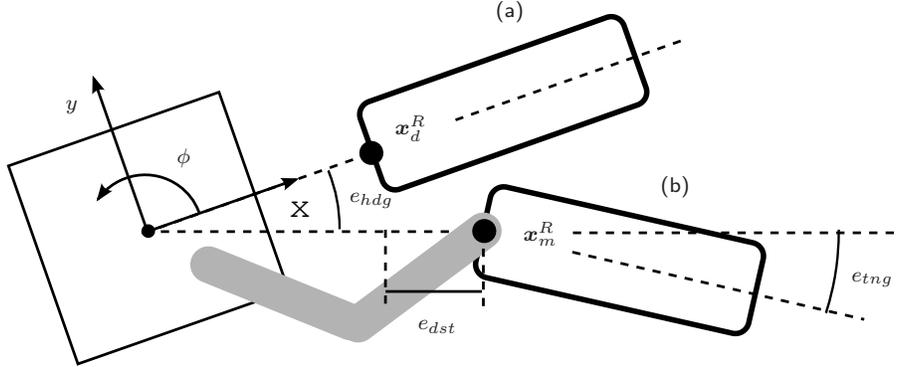
Figure 10: (a) Desired and (b) actual configuration of the base w.r.t. the object, described by a desired and measured pose of the manipulator’s end-effector,  $\mathbf{x}_d^R$  and  $\mathbf{x}_m^R$  respectively.
