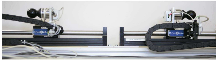
Fig. 4.24: 1DoF experimental setup consisting of two identical linear direct drive actuators, Thrusttube modules ME2504 from Copley Controls Corp..
