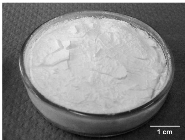
Fig. 6. Optical image of a  $\text{MgCO}_3$  aerogel sample obtained after supercritical drying.
