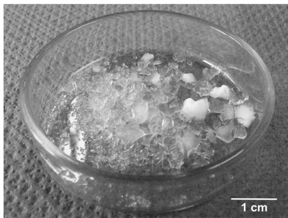
Fig. 4. Optical image of a  $\text{MgCO}_3$  xerogel sample after drying under ambient conditions; grid  $0.5\text{ cm}$ .
