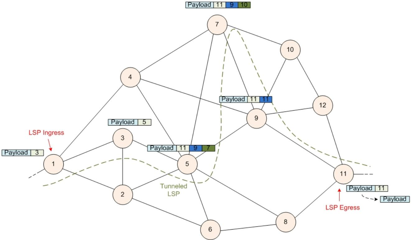
**Fig. 4.8:** Example of an LSP in which the packets enter a double tunnel at node 5
