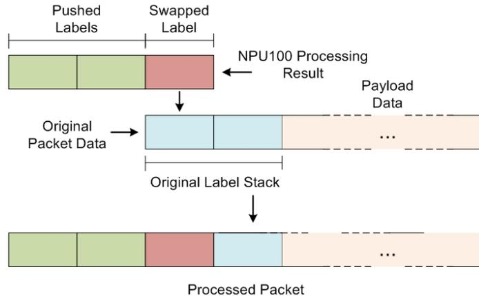
**Fig. 4.10:** Example Packet Reassembly in a Swap, Push, Push Scenario
