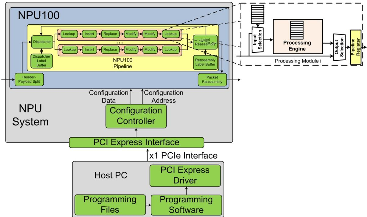
**Fig. 3.14:** Block Diagram of the NPU100 Configuration Architecture
