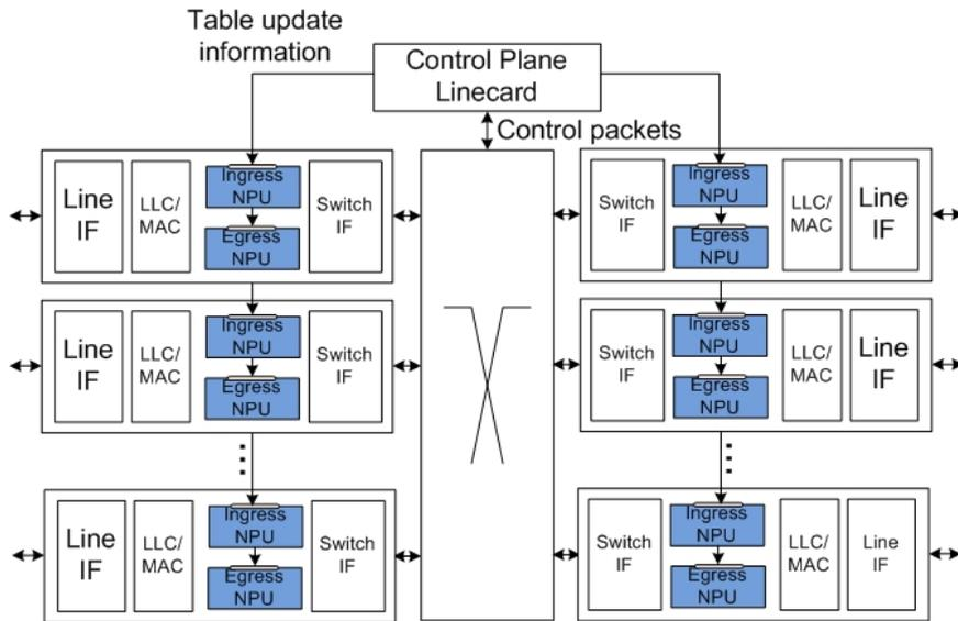
**Fig. 2.8:** Overview of an Example 100 Gbit/s CGE Node Architecture
