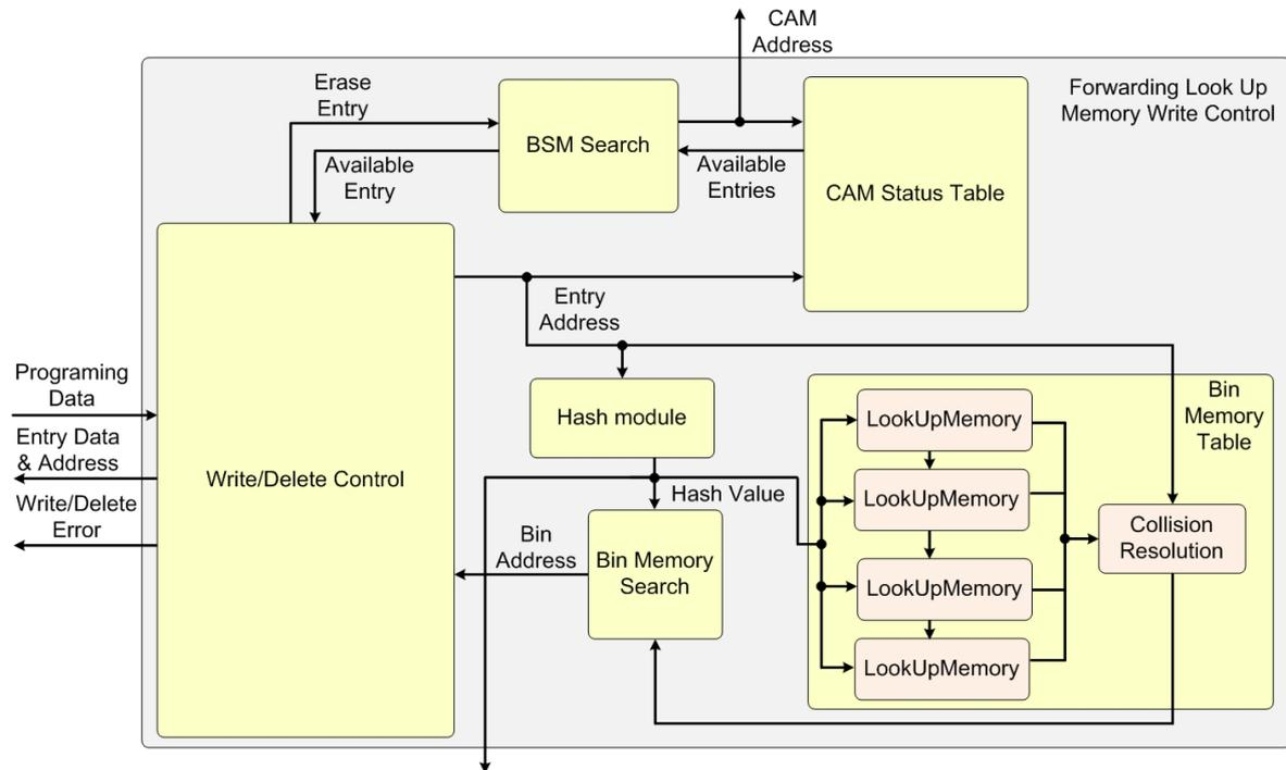
**Fig. 4.26:** Block Diagram of the Forwarding Lookup Write Control Architecture
