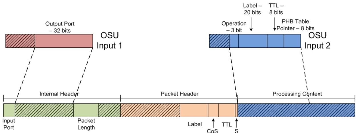
**Fig. 4.20:** Example of the Processing Results Being Reinserted into the Pipeline Word by the OSU
