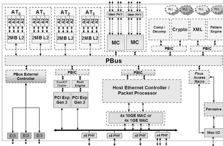
Fig. 2.10: Block Diagram of the New Generation IBM NPU [37]
