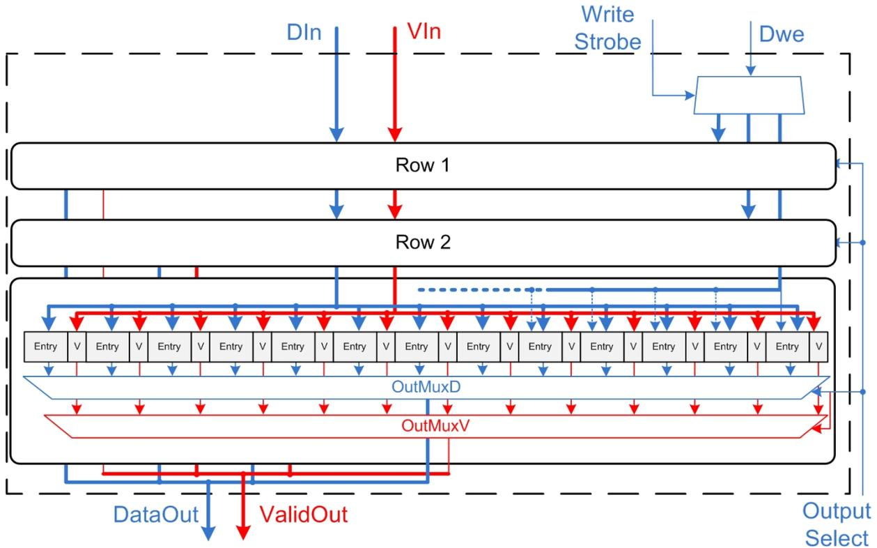
**Fig. 4.16:** Overview of the Buffer Design for Three Mini Pipelines and Thirteen Mini Pipeline Stages
