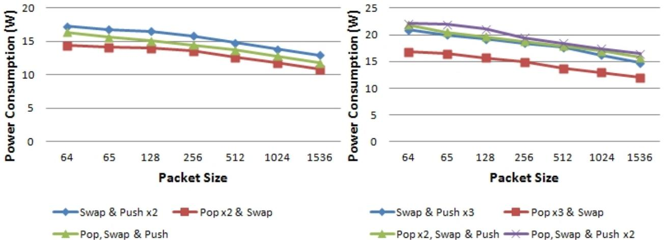
**Fig. 5.5:** Dynamic Power Consumption per Packet Size for Loop Run Scenarios Three and Four
