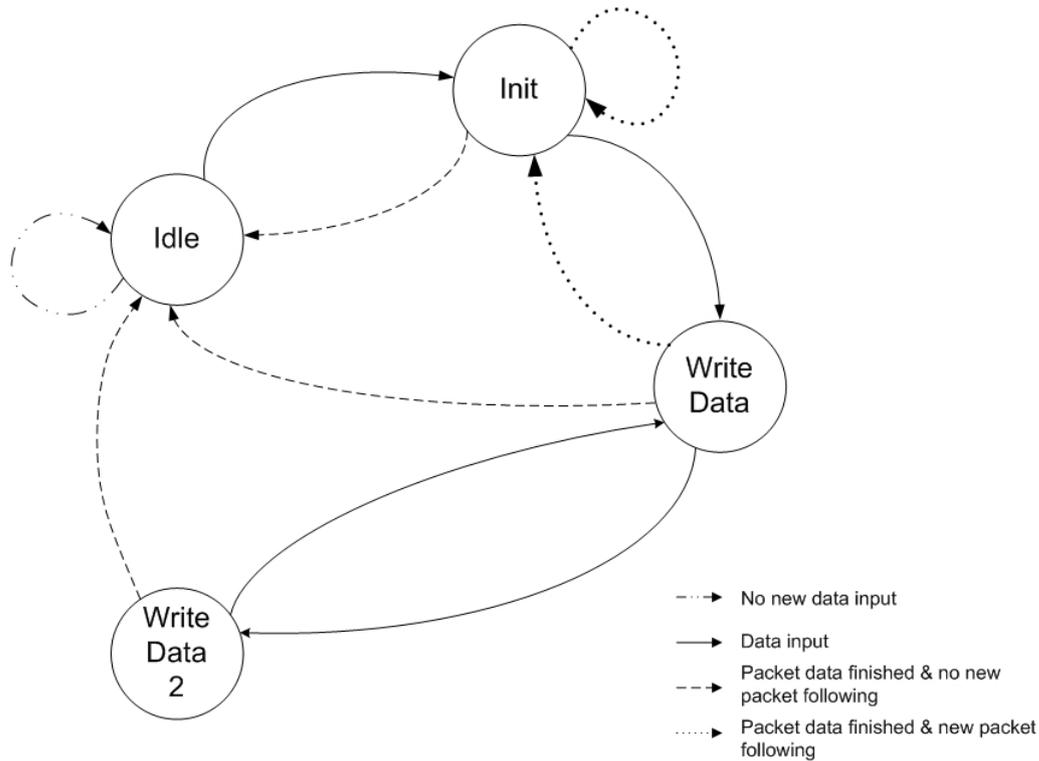
**Fig. 4.4:** State Diagram of the Header-Payload Split Module. Solid Lines Show Transitions During Data Input, Dashed Lines Transitions when a Packet is Finished and no New Packet is to Start in the Following Clock Cycle and Dotted Lines transitions when a Packet is Finished and is Trailed by a New Packet in the Next Clock Cycle.
