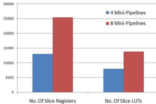
**Fig. 5.11:** Dispatcher and Label Reassembly Module Resource Consumption for 4 and 8 Mini-Pipelines
