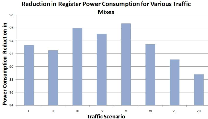
**Fig. 3.10:** Registered Architecture Dynamic Register Power Consumption Reduction Relative to the Conventional Pipeline
