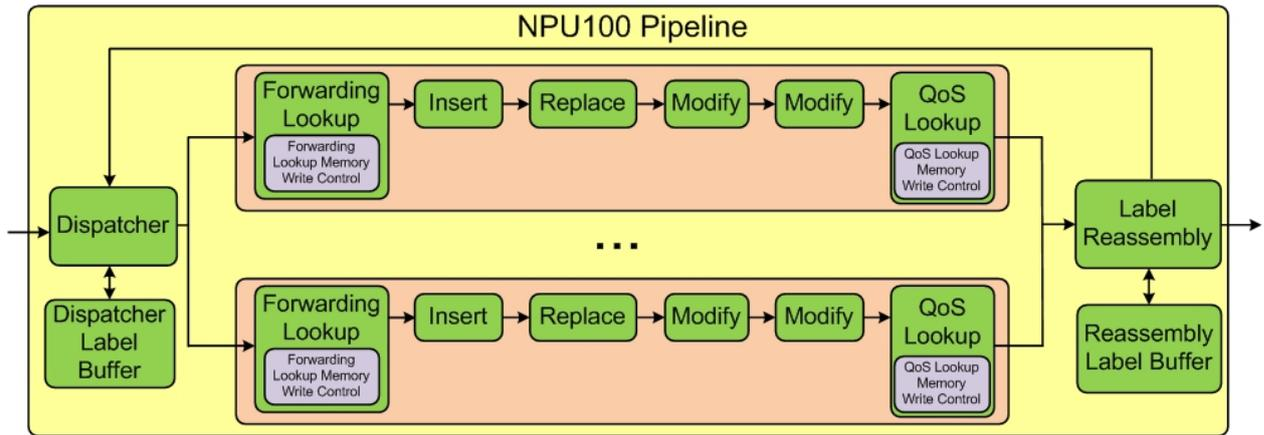
Fig. 3.13: Folded Pipeline Architecture Modelled in xPower
