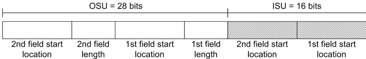
**Fig. 4.21:** Microcommand Table Entry Structure for the ISU and OSU
