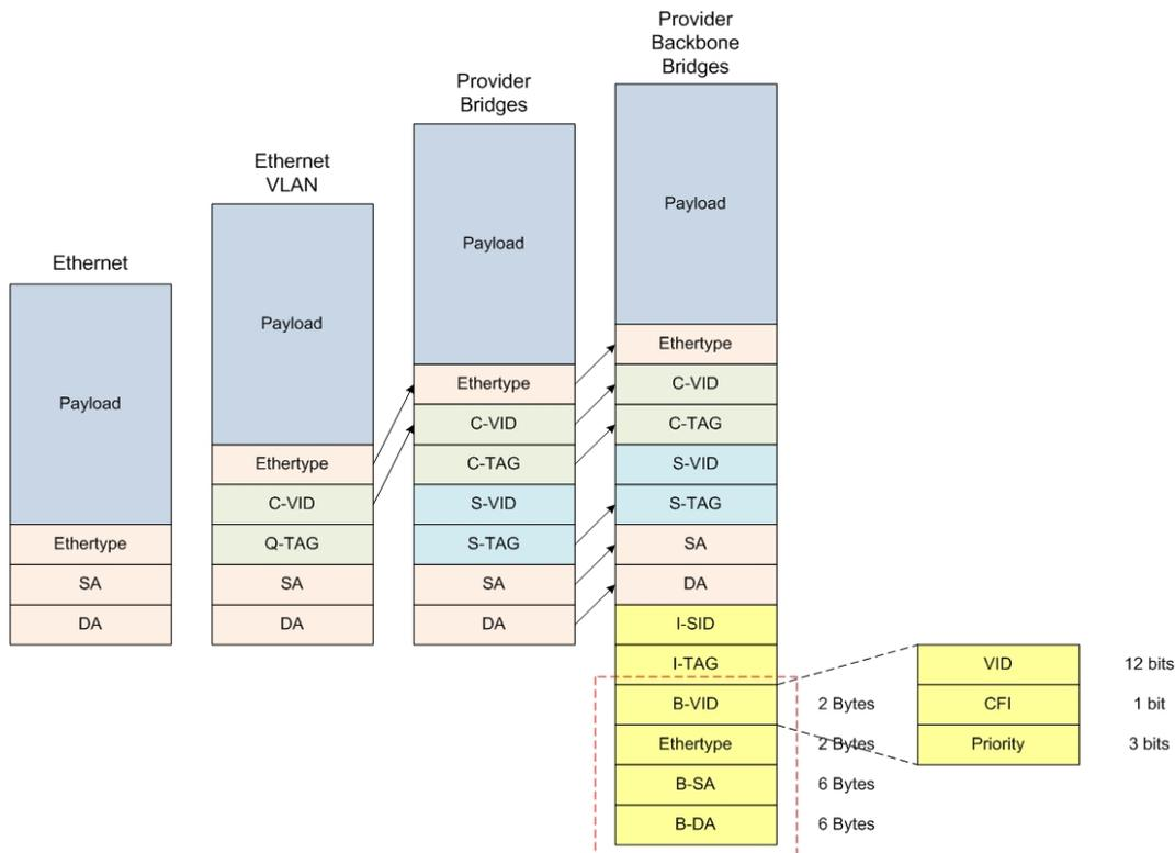
**Fig. 2.6:** Overview of the PBB-TE Frame Development over the Years
