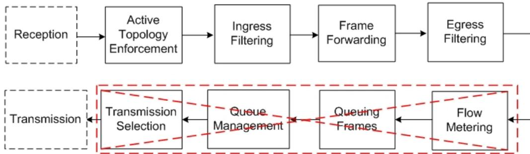
**Fig. 2.7:** Processing Steps Required by a PBB-TE Frame
