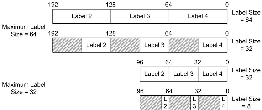
**Fig. 4.13:** Dispatcher Label Buffer Input Vector for Various Values of the Maximum Label Size Generic and the Actual Label Size Currently Being Processed in the Pipeline
