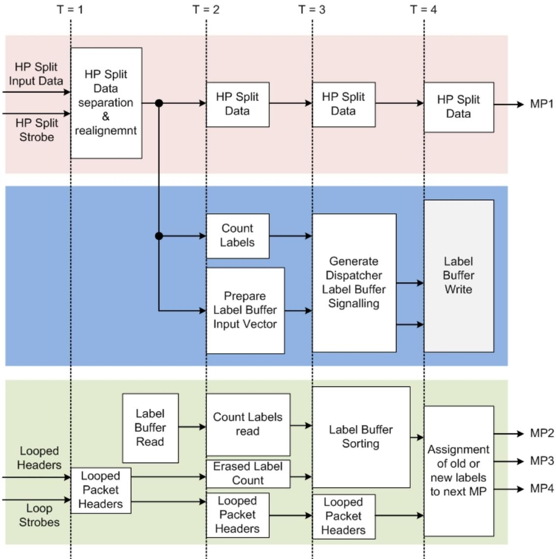
**Fig. 4.12:** Overview of the Dispatcher Design, Showing the Three Parallel Pipelines which Make up the Module
