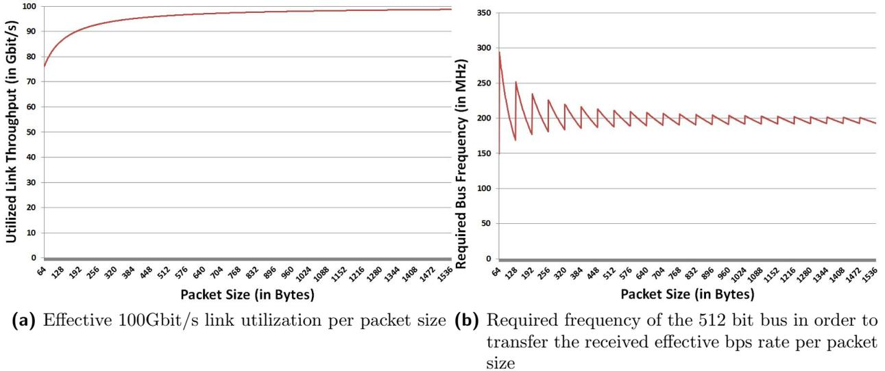
**Fig. 4.2:** Utilized Link Throughput and Required NPU100 Internal Bus Frequency per Packet Size
