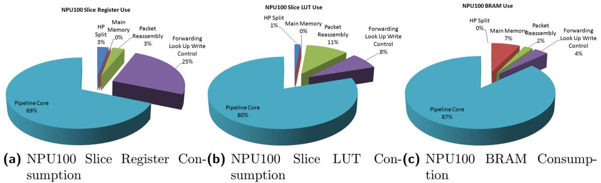
**Fig. 5.1:** Resource Use Break Down between the Various NPU100 Modules
