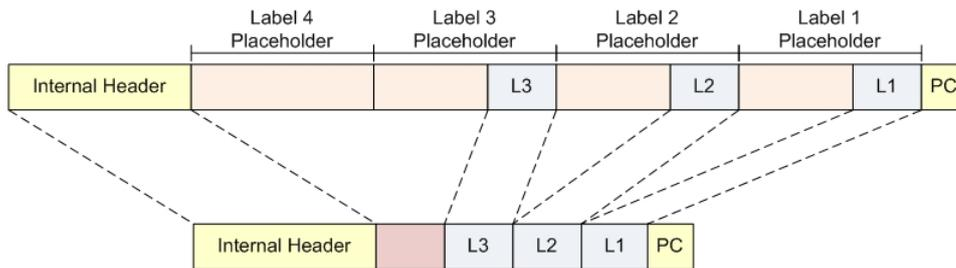
**Fig. 4.6:** Header Alignment Process Example in the Packet Reassembly Module
