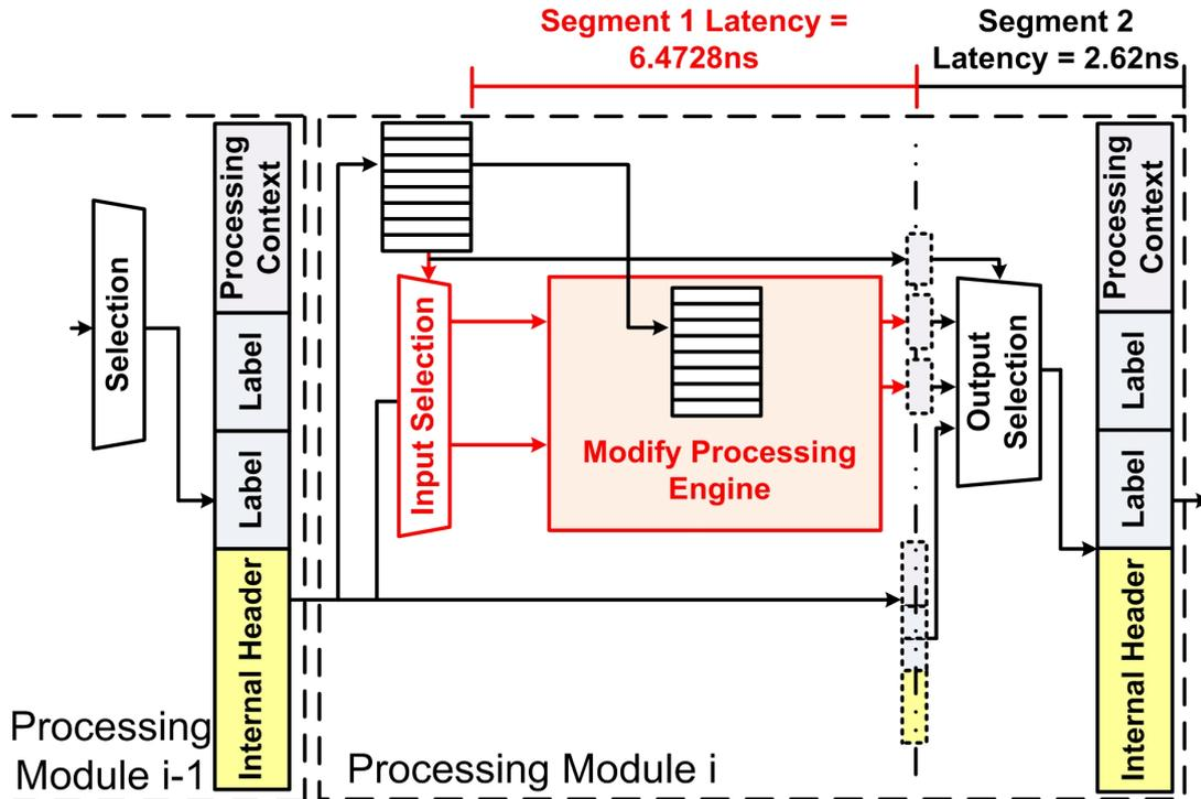
**Fig. 5.9:** Reduction of the Critical Path by Pipelining
