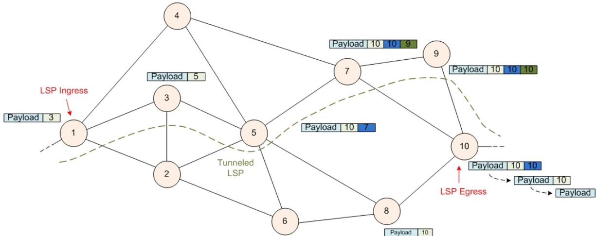
**Fig. 2.4:** Example of an MPLS-TP LSP with two Tunneling Layers
