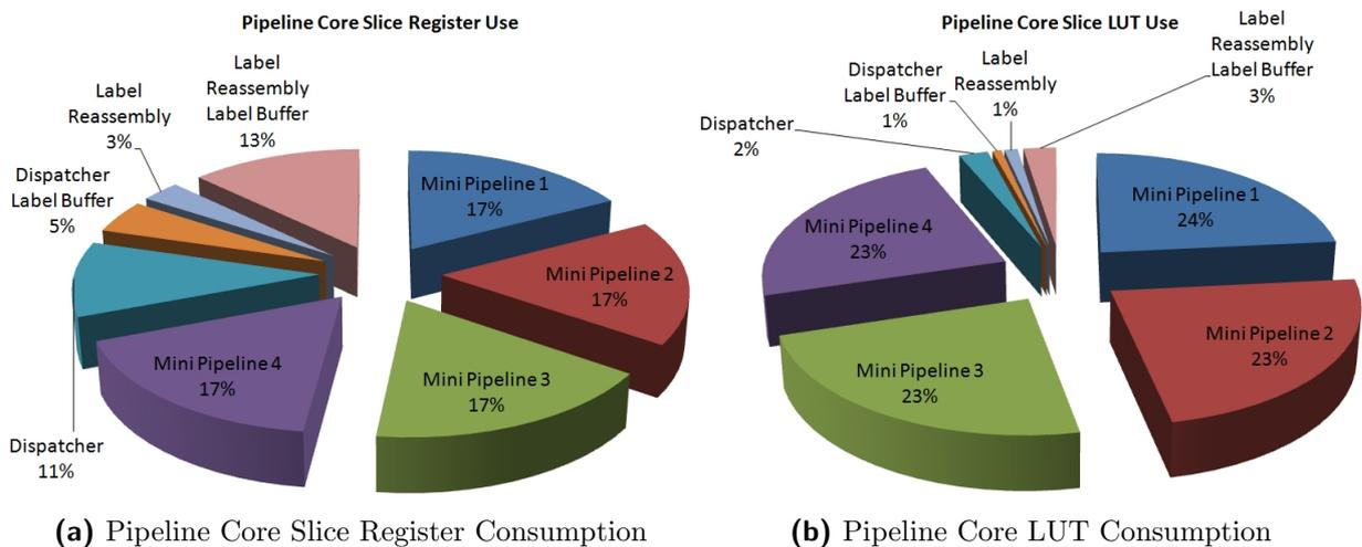
**Fig. 5.2:** Resource Use Break Down between the Various Pipeline Core Modules
