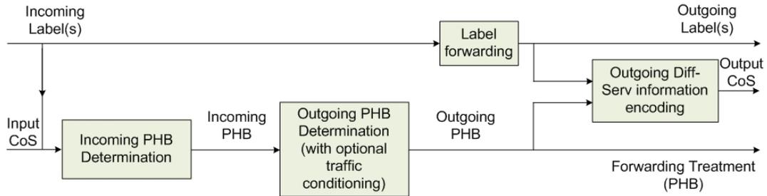
**Fig. 2.2:** Overview of the MPLS Forwarding Process
