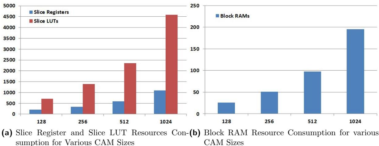
**Fig. 4.25:** FPGA Resource Consumption for Various CAM Sizes
