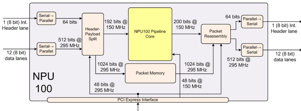
**Fig. 4.1:** Overview of the Architecture of the NPU100 Outer Layer with Bus Widths and Operating Frequencies
