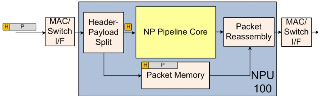
**Fig. 3.2:** Block Diagram of the NPU100 Outer Layer, which Shows how the Header is Copied and Sent to the Pipeline core while the Complete Packet is Stored in the Packet Memory.
