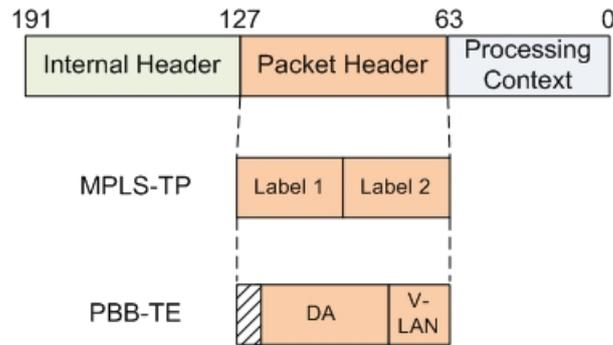
**Fig. 3.8:** General NPU100 Pipeline Word Structure, along with MPLS-TP and PBB-TE Variants
