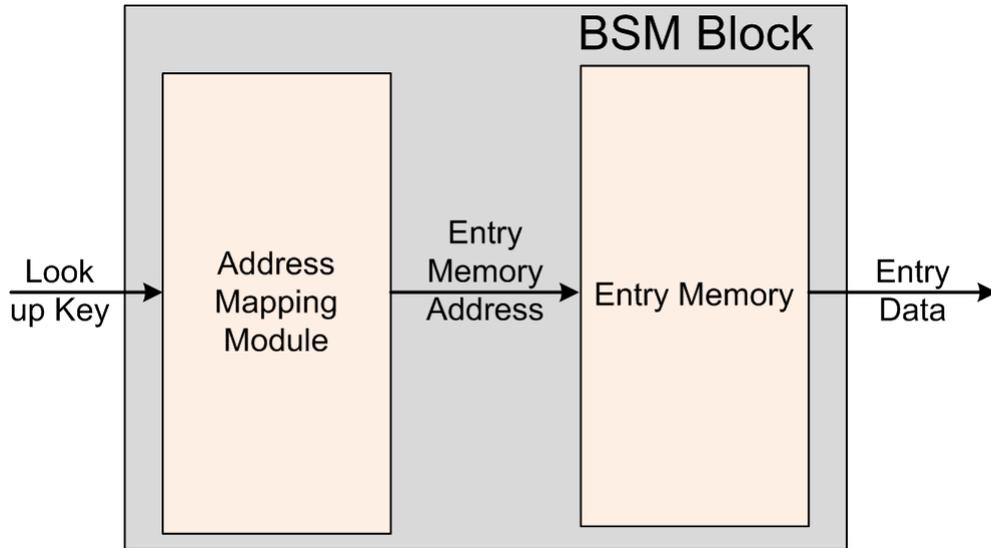
**Fig. 4.24:** Block Diagramm of the Black Sheep Memory Block
