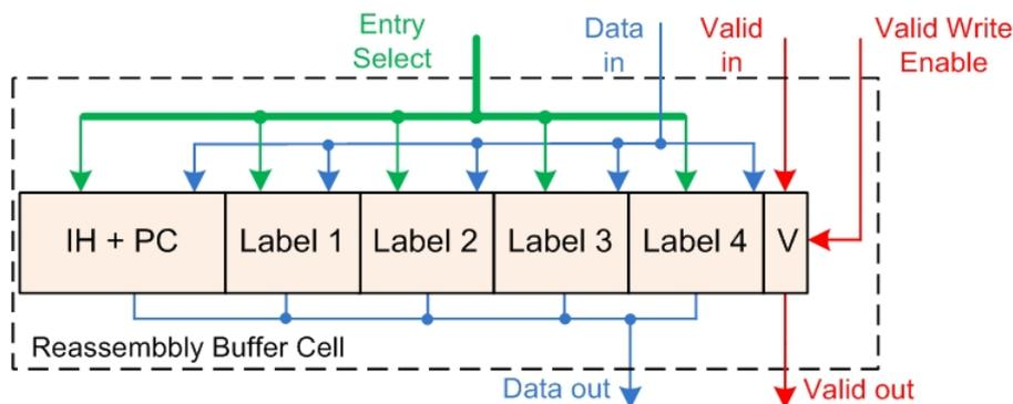
**Fig. 4.17:** Reassembly Buffer Cell Block Diagram
