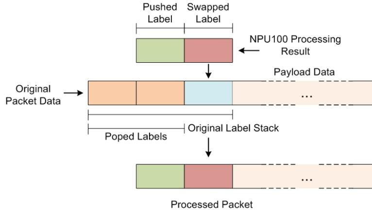
**Fig. 4.9:** Example Packet Reassembly in a Pop, Pop, Swap and Push Scenario
