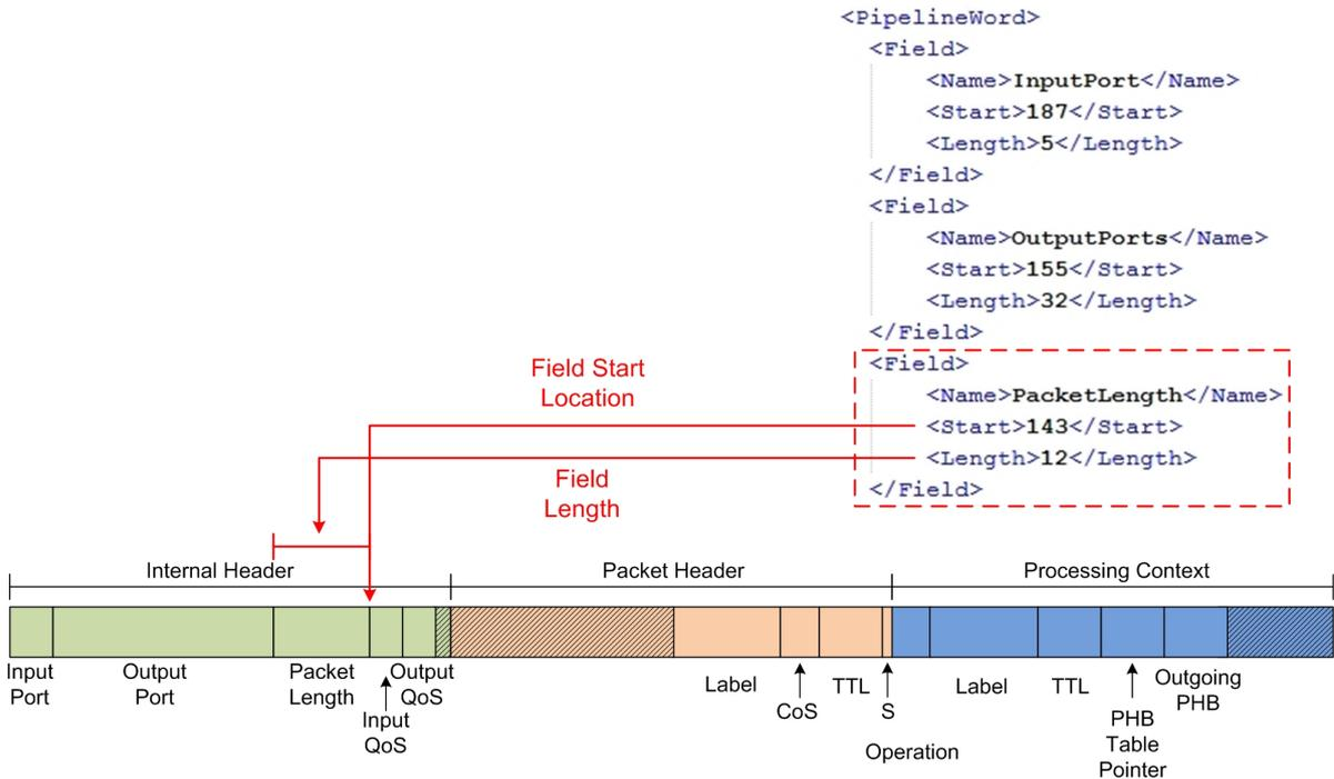
**Fig. 4.31:** Example of the Definition of a Field in the PIF
