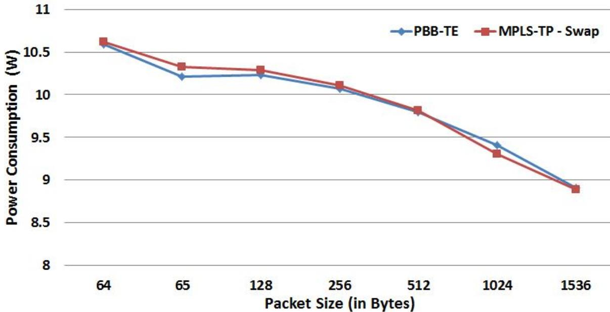
**Fig. 5.7:** Dynamic Power Consumption per Packet Size for PBB-TE Processing
