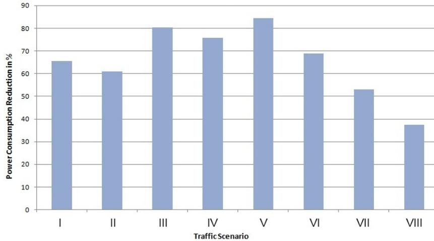
**Fig. 3.9:** Folded Architecture Dynamic Register Power Consumption Reduction Relative to the Conventional Pipeline
