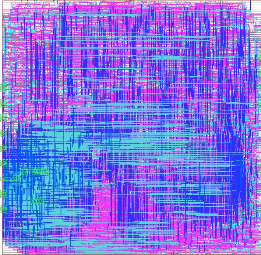
**Fig. 5.10:** Die Shot of a Fully Routed Modify Module
