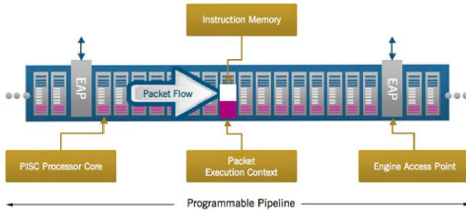
**Fig. 2.14:** Overview of the DataFlow Architecture used in the Xelerated NPs [62]
