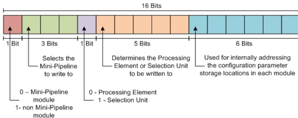
**Fig. 4.29:** NPU100 Configuration Addressing
