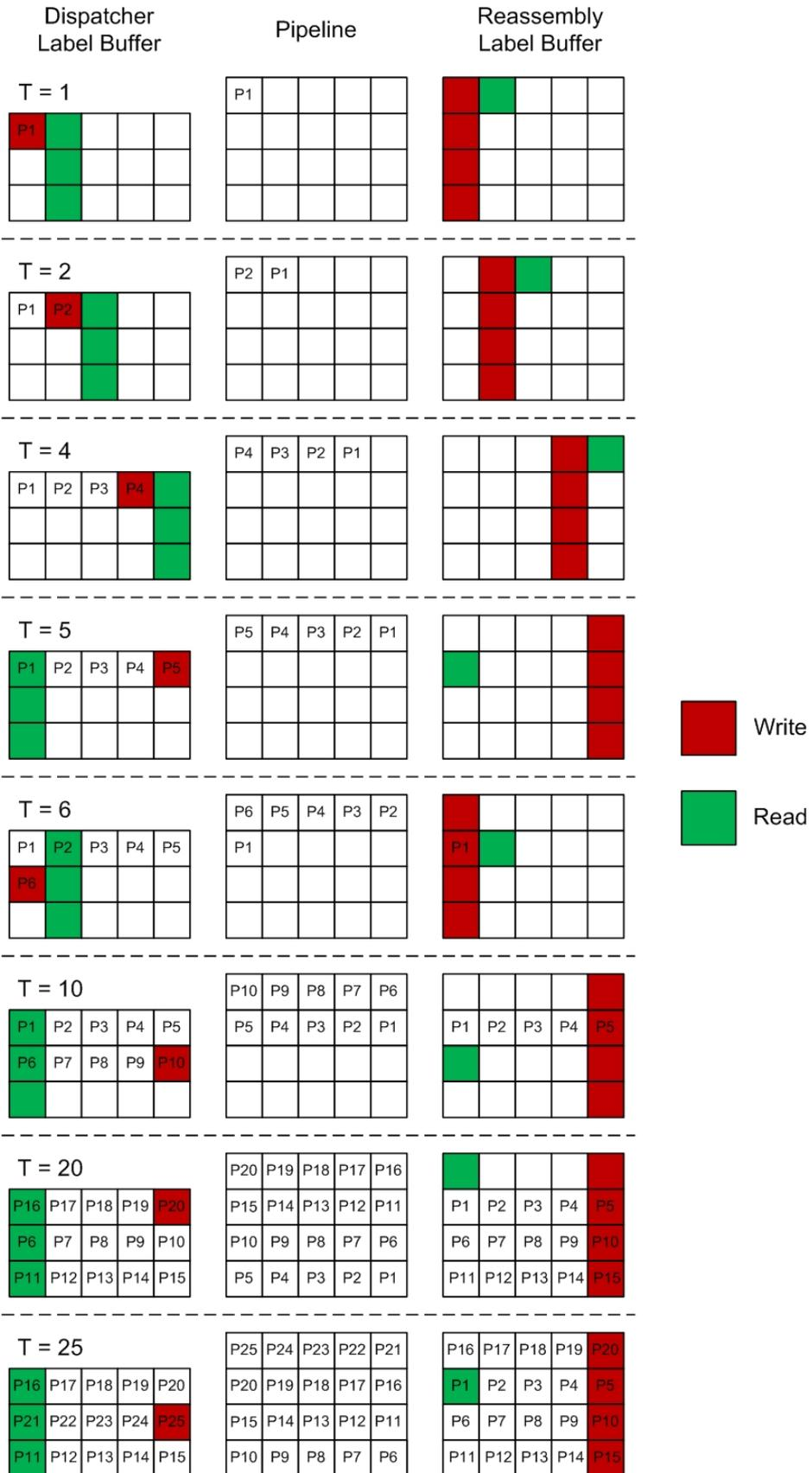
Fig. 4.15: Overview of the Label Buffer Time Slot Concept
