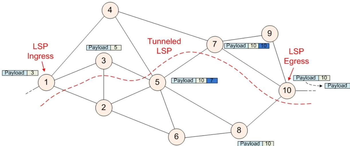
**Fig. 2.3:** Example of an MPLS-TP LSP with one Tunneling Layer
