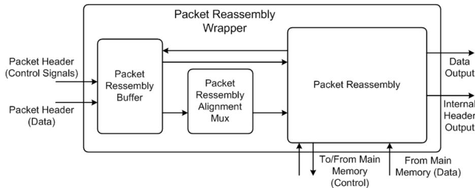
**Fig. 4.5:** Packet Reassembly Submodule Block Diagram
