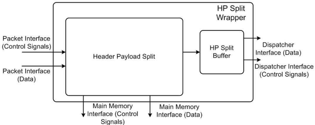
**Fig. 4.3:** Overview of the Header Payload Split Submodule
