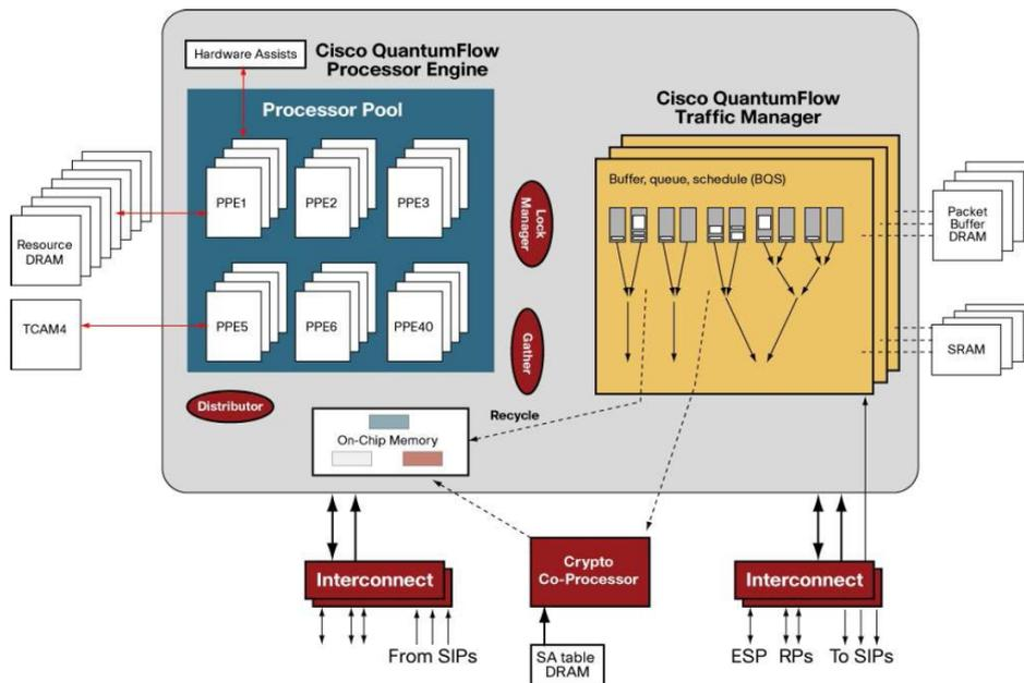
**Fig. 2.12:** Architectural Overview of the Cisco ASR 1000 Embedded Services Processor [24]
