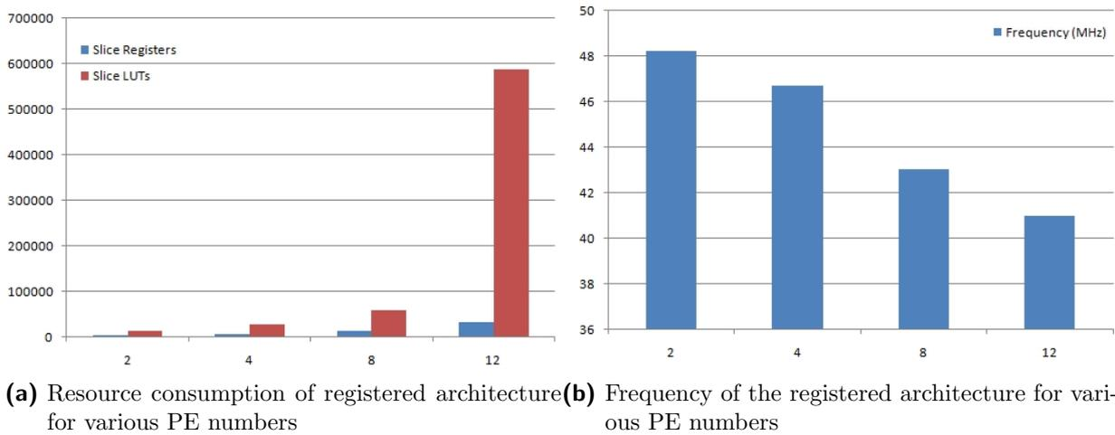
**Fig. 3.12:** Registered Architecture Resource Consumption and Frequency for Various PE Numbers
