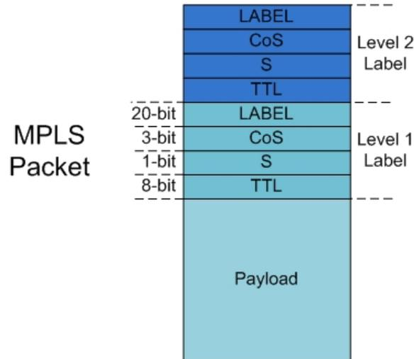
**Fig. 2.1:** MPLS Label Field Structure
