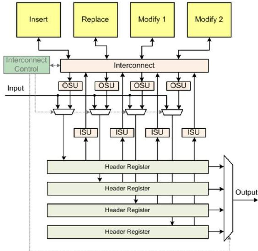
Fig. 3.11: Implementation of a Registered Architecture Prototype
