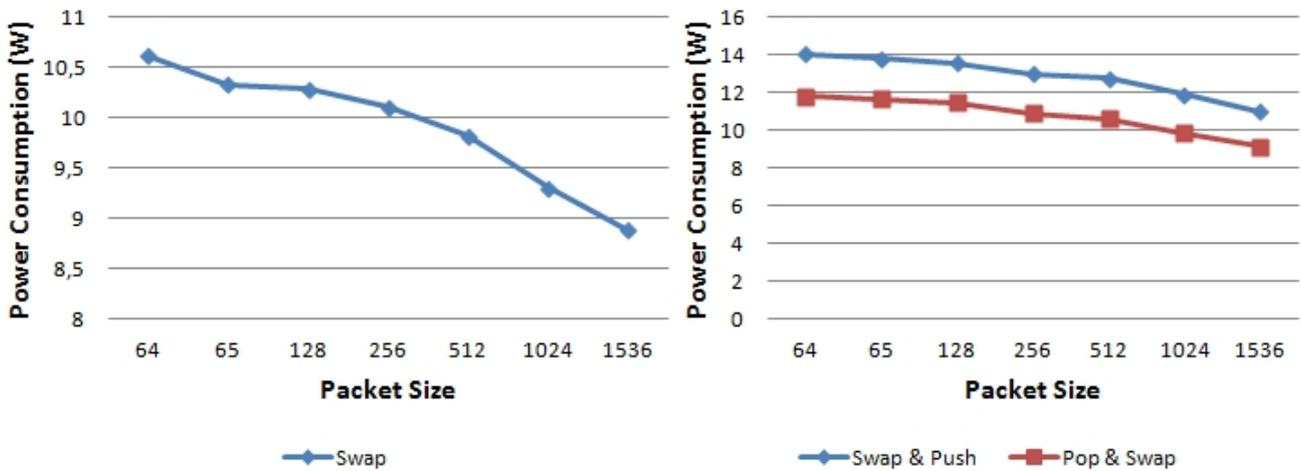
**Fig. 5.4:** Dynamic Power Consumption per Packet Size for Loop Run Scenarios One and Two
