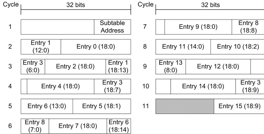
**Fig. 4.37:** Allocation of QoS Subtable Entry Words to Programming Words
