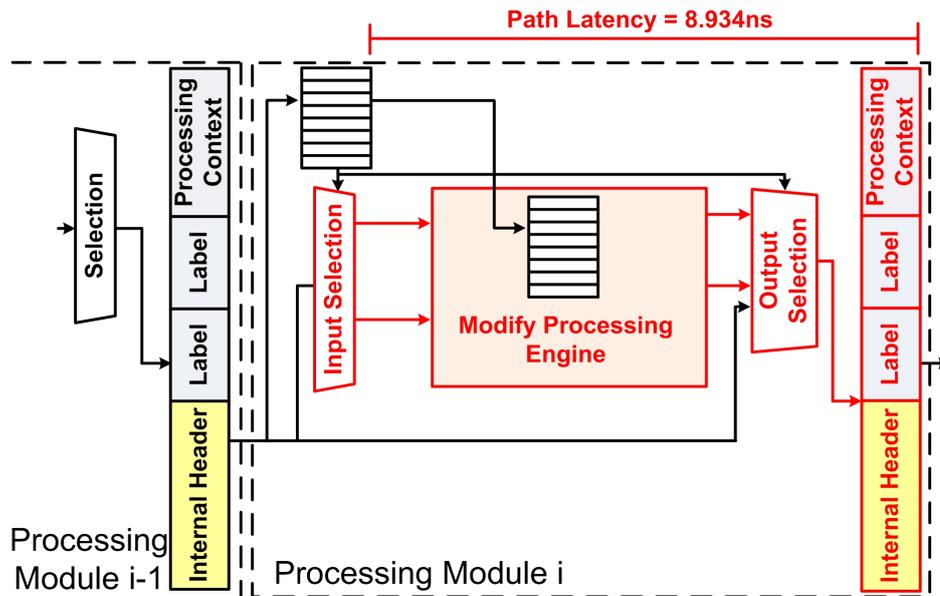
**Fig. 5.8:** Critical Path Constraining the Performance of the NPU100
