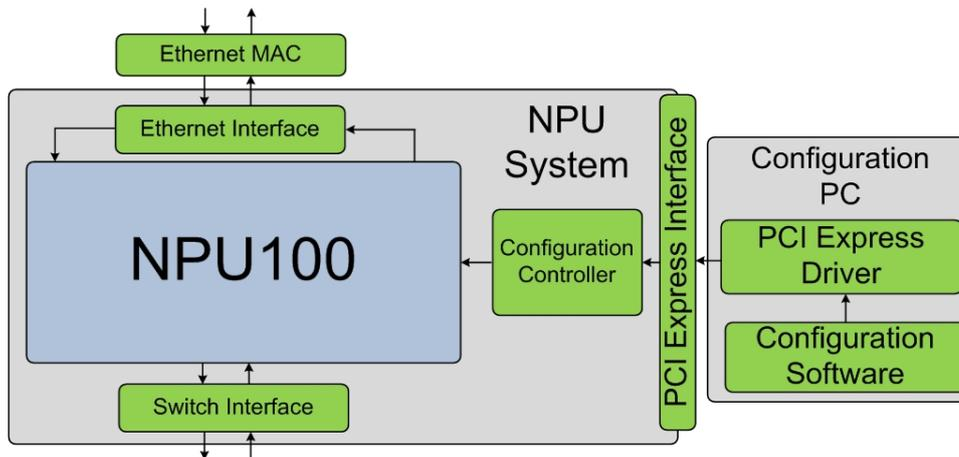
**Fig. 3.1:** High-level Block Diagram of the NPU100 System
