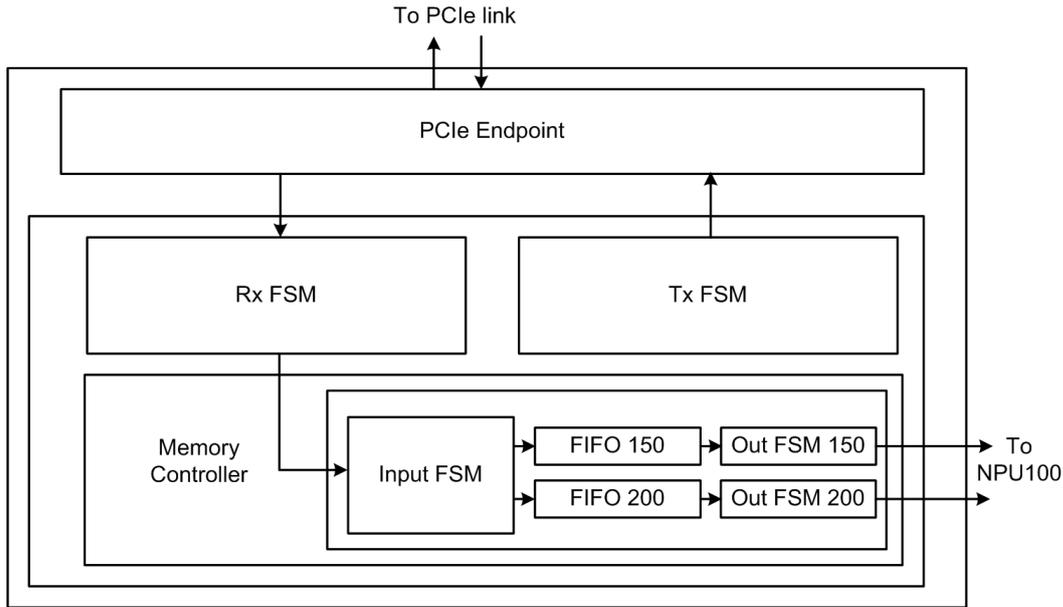
**Fig. 4.30:** Block Diagram of Hardware Modules Making Up the PCI Express Interface
