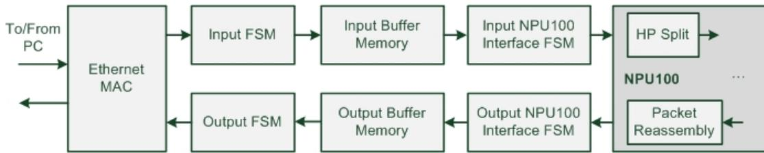
**Fig. 5.13:** Ethernet Interface Module Chain Block Diagram
