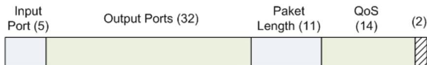
**Fig. 3.3:** Structure of the NPU100 Internal Header
