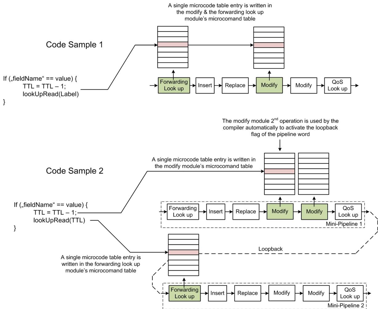
**Fig. 4.36:** Example of Statement Mapping to PEs with the MP Loop Being Used
