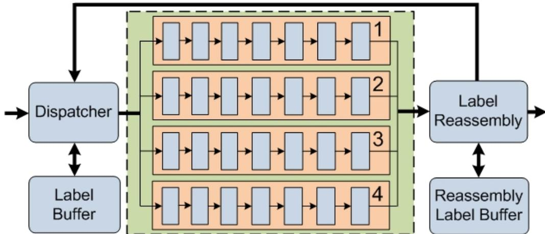
**Fig. 3.6:** Block Diagram of the Folded Pipeline Architecture
