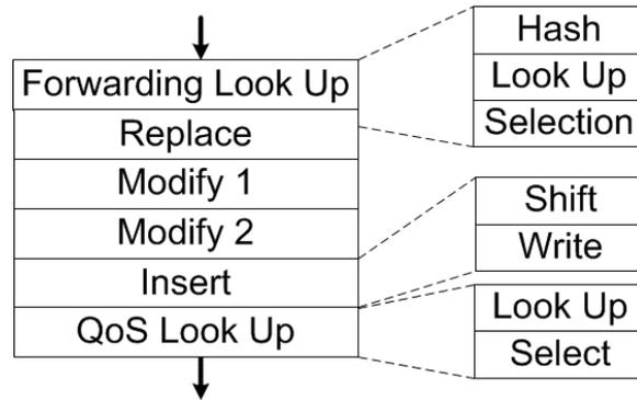
**Fig. 3.7:** NPU100 Mini-Pipeline Stages Derived from CGE Protocol Requirements
