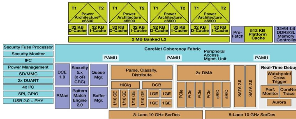
**Fig. 2.11:** Block Diagram of the Freescale QorIQ AMP Series T2080 Communications Processor
