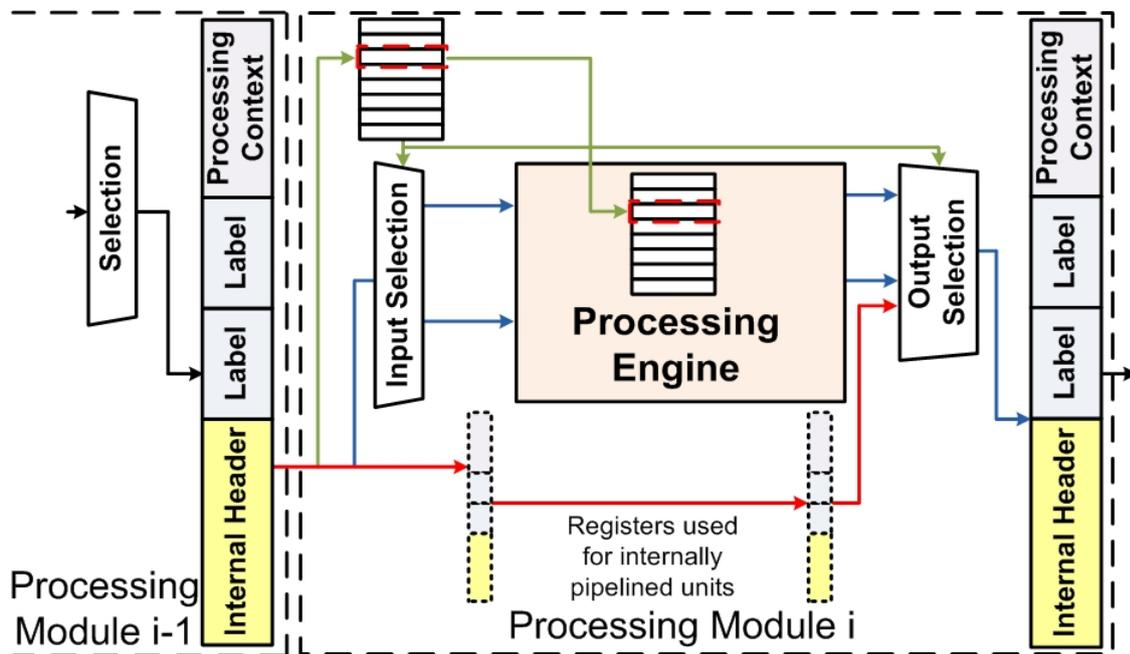
**Fig. 4.19:** ISU bit Selection and Field Extraction, Followed by the Processing of Data in the PE and Recombination of Processing Results and Original Register Data in the OSU
