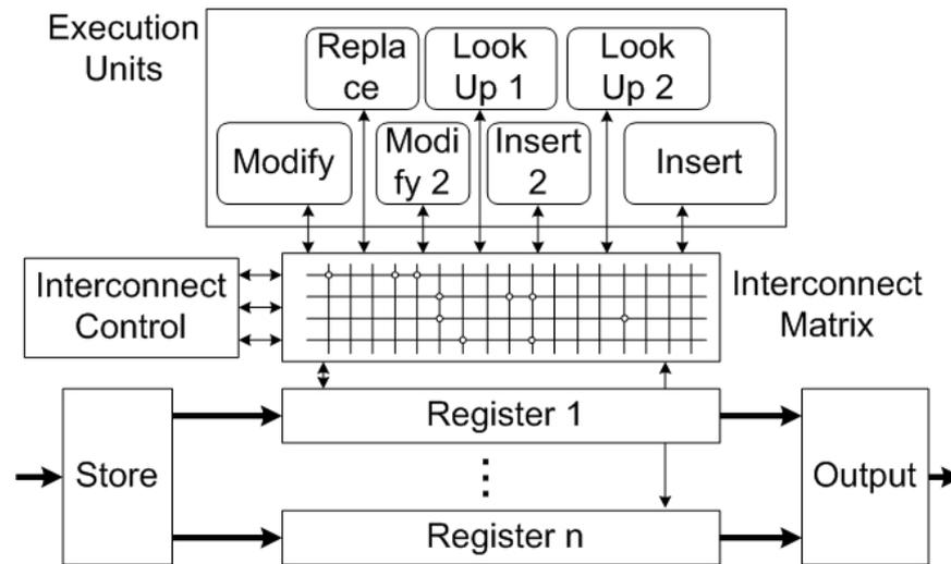
Fig. 3.5: Block Diagram of the Registered Architecture
