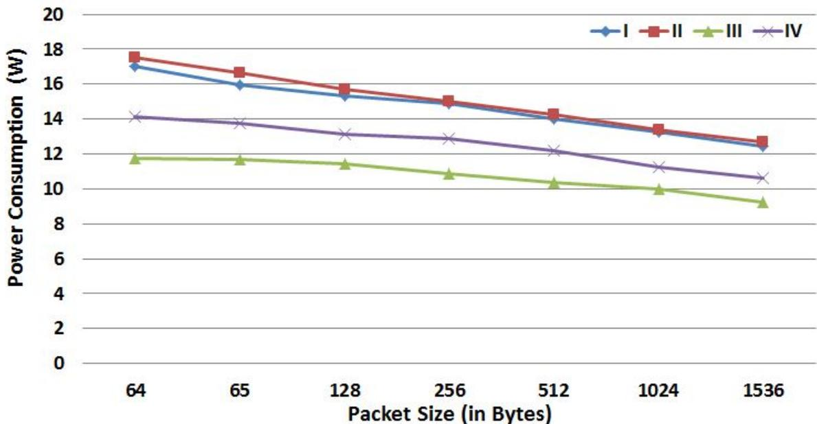
**Fig. 5.6:** Dynamic Power Consumption per Packet Size for Traffic Scenarios I through IV as Detailed in Table 5.3
