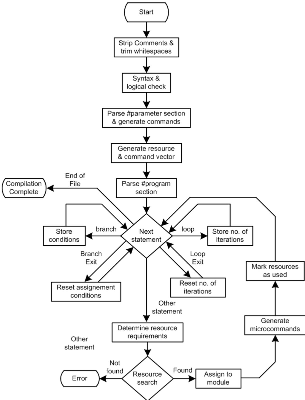
**Fig. 4.33:** Flow Diagram of the CPF Compilation Process
