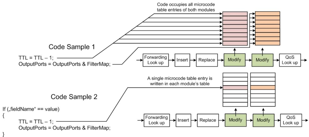
**Fig. 4.35:** Further Examples of Different Task Allocation to the PEs
