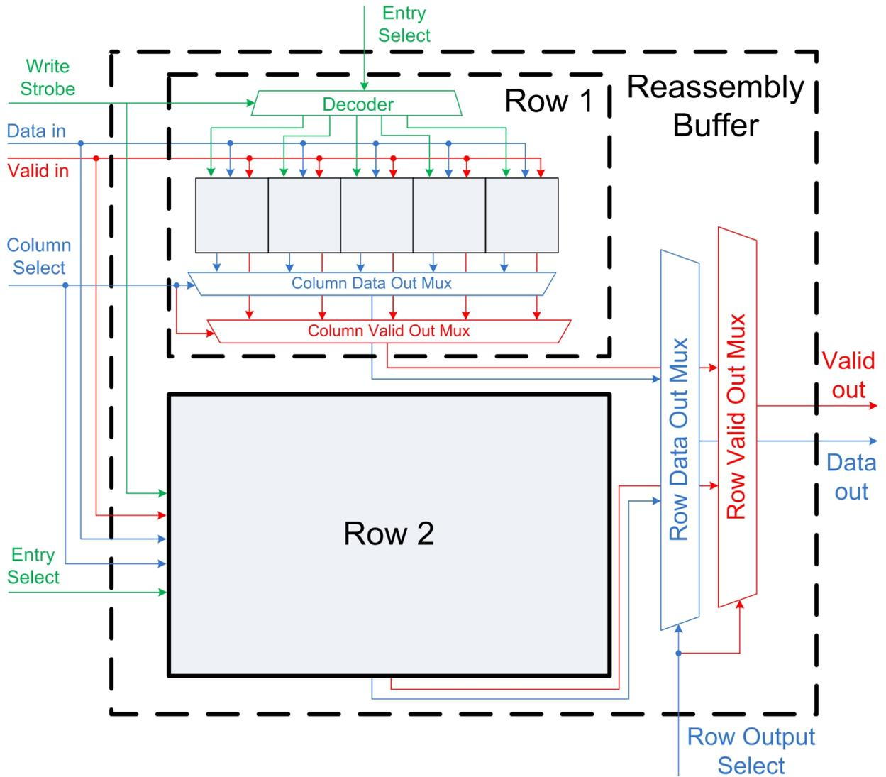
**Fig. 4.18:** Overview of the Reassembly Buffer Structure for Two Minipipelines and Five Stages per Mini Pipeline
