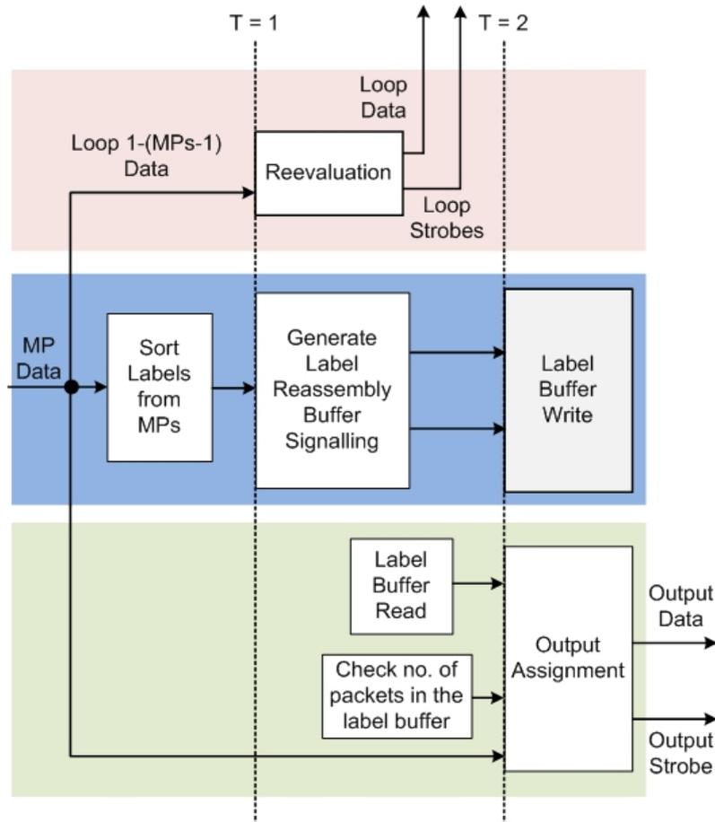
**Fig. 4.14:** Overview of the Label Reassembly Design with the Three Parallel Pipelines Demarcated
