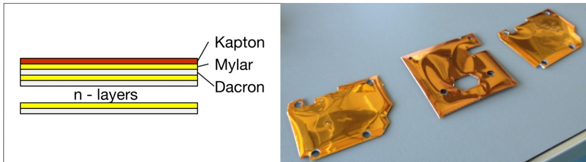
Figure 4-17: left) principle layout of a MLI blanket and right) MLI blanket of a cubesat.
