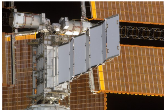
Figure 4-16: Radiators with ammonium working fluid, on the International Space Station (NASA 2012b).
