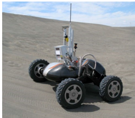
Figure 2-5: The SCARAB Rover concept. A 1:1 scale engineering model in field tests (Wettergreen et al. 2010).
