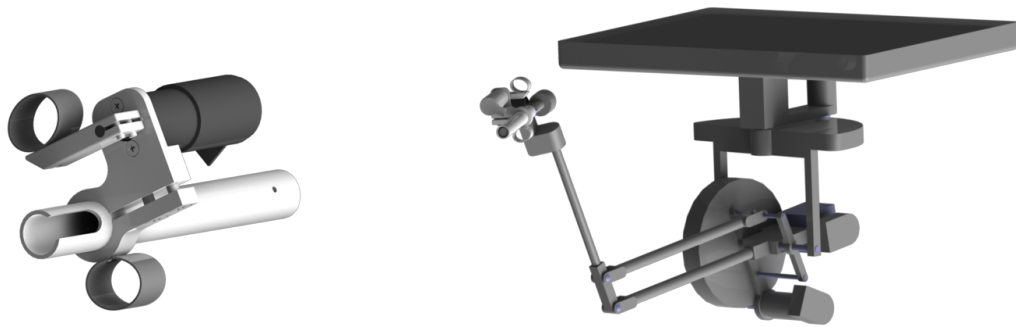
Figure 5.3: Continuous input handle (left) and mounted handle on Phantom™ device (right).
