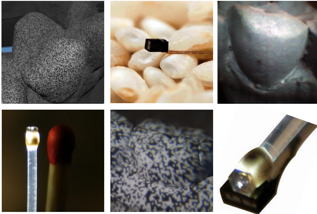
Figure 6.1: Development of miniaturized camera setup, from left to right: simulated camera image, NanEye™ micro camera [image courtesy of Awaiba GmbH], dental scene captured with micro camera, developed micro projector, pattern projected on dental scene, and final setup.
