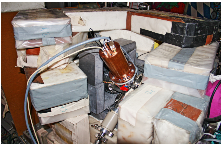
Figure 3.26: The HXR detector vessel is properly shielded against the neutrons and stray \gamma -rays in the ASDEX hall, by the lead bricks (inner-wall) and paraffin wax bricks (outer-wall).
