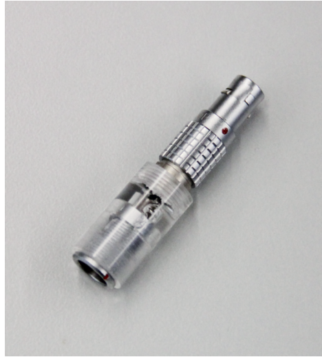
Figure 3.8: The noise proof LEMO adapter found to be responsible for picking up noise in tokamak environment.
