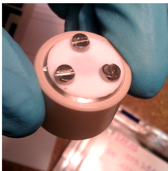
Figure 3.15: The scintillator holder cap. The steel part holds the scintillator crystal. The outer ceramic part holds both the SDD and the steel cap together rigidly.
