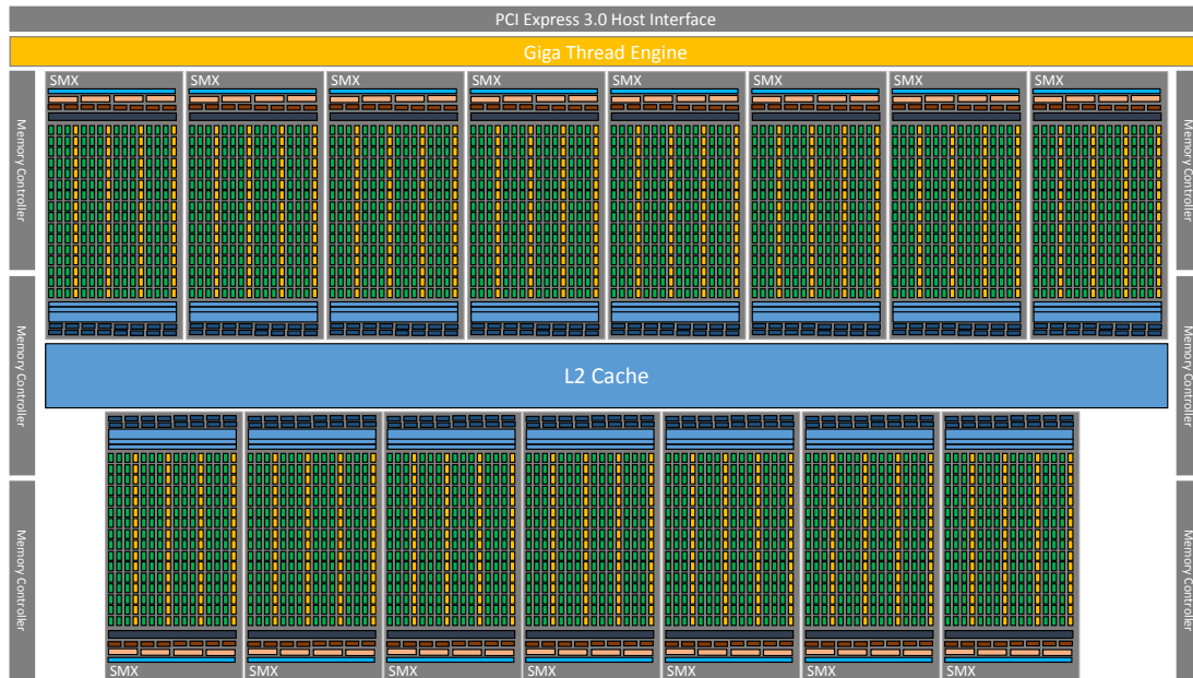
Figure 2.4: Block diagram of an NVIDIA GPU with Kepler GK110 architecture (according to [NVI12d], adapted). The chip offers up to 2880 CUDA cores for single-precision arithmetic, 960 for double-precision, 480 for transcendental operations and 480 for memory loads and stores. The number of available cores varies between products.
