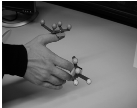
Fig. 2. IRTTs mounted at user's fingers
