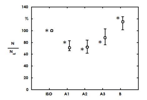
Figure 1-Loudness of pass-by sounds from a passenger car at 50 km/h in 7.5 m distance for a "normal" tire on different road surfaces. ISO represents the ISO10844 road surface; A1, A2, A3 stand for three different sound absorbing road surfaces, and B for a conventional, nonabsorbing road surface. Data from psychoacoustic experiments (circles) in comparison to physically measured values of percentile loudness N<sub>5</sub> (stars)
