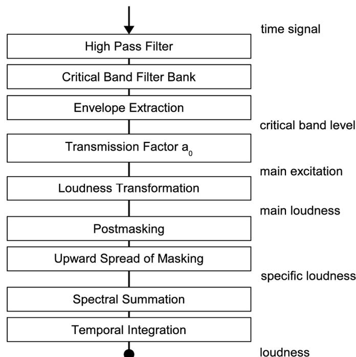
Fig. 1. Block diagram of the Dynamic Loudness Model DLM (after Chalupper and Fastl 2002).
