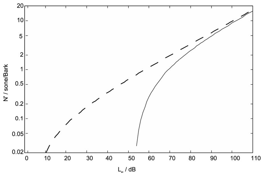
Fig. 2. Loudness transformation for normal hearing persons (dashed) and a person with 50 dB hearing loss and recruitment (solid) (after Chalupper 2002)
