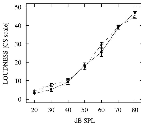
Figure 1: Calibration curves: Loudness functions for identical samples of pink noise obtained from the two groups of subjects ( $N = 20$  each) judging the original (filled circles) and neutralized (diamonds) sounds.
