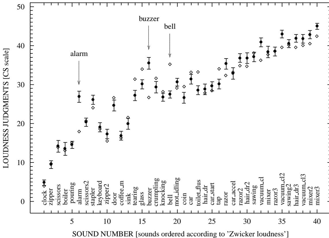
Figure 3: Loudness judgments of the 40 test sounds (labelled along the abscissa) in their original (filled circles) and neutralized (diamonds) version. Variability is indicated for the original condition only by plotting the data points plus/minus one standard error of the mean; in the neutralized condition it is of comparable magnitude.
