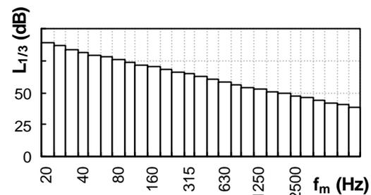
**Fig. 1:** Third-octave band spectrum of the basic stimulus, simulating a typical spectrum inside high-speed trains.
