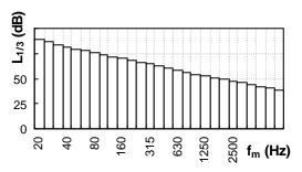
**Fig. 1:** Third-octave band spectrum of the basic stimulus, simulating a typical spectrum inside high-speed trains.
