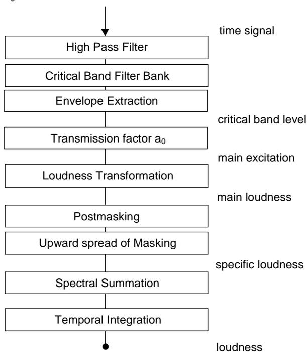
**Figure 3:** Block diagram of the Dynamic Loudness Model (DLM) proposed by Chalupper and Fastl 2002.
