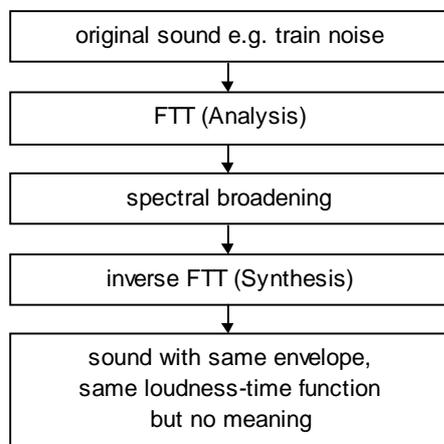
**Figure 4:** Block diagram illustrating the procedure to neutralize the meaning of sound.
