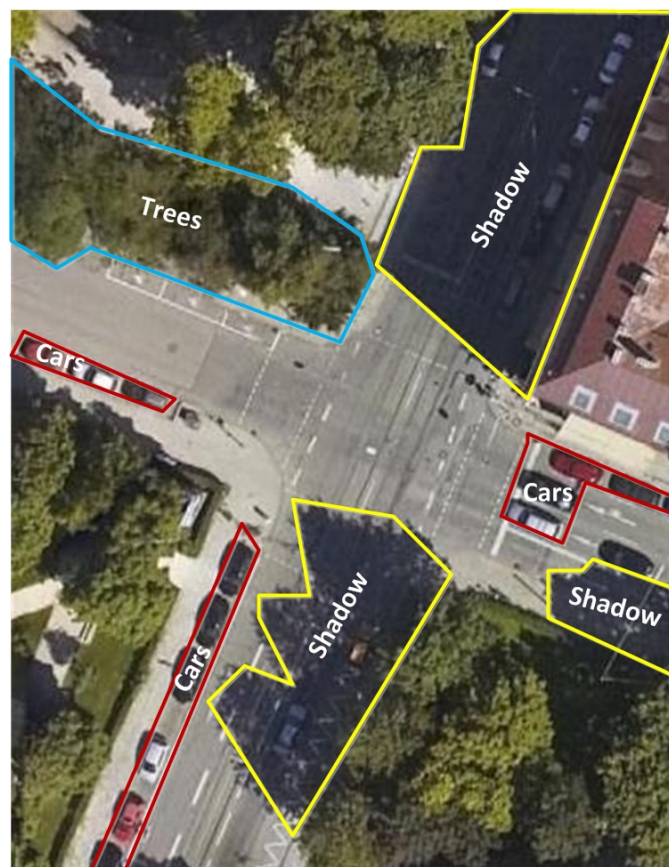
Fig. 2-5 A typical image with roads as low-level objects at a intersection
