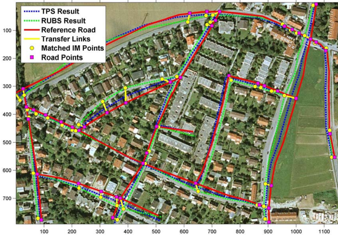
Fig. 5-18 Transformed road network with links to additional end nodes from extracted features in test area 1
