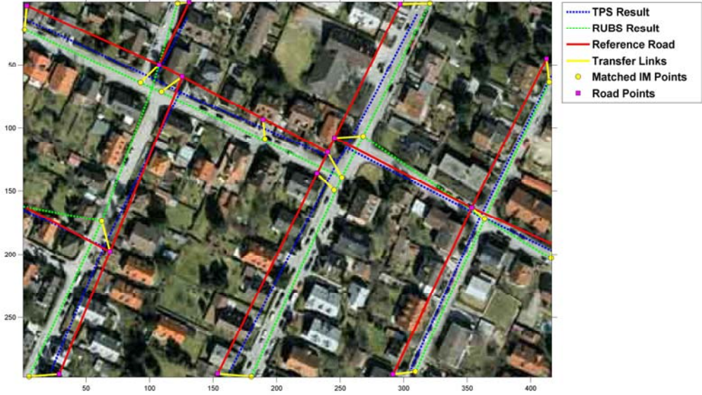
Fig. 5-20 Transformed results in test area 3
