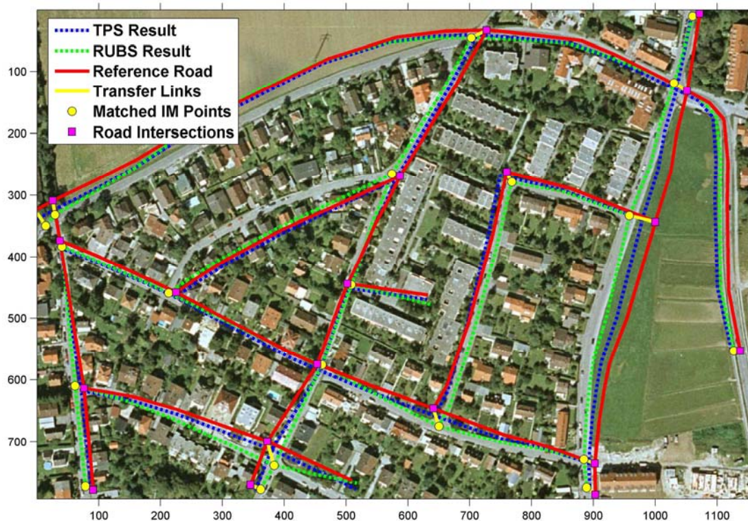
Fig. 5-17 Transformed road network with the matched points in test area 1 (Image Point, IM)
