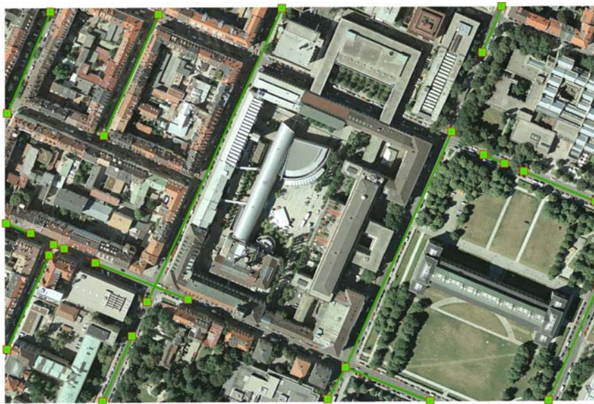
Fig. 2-8 The unreliable topology of the extracted road lines (the green lines)
