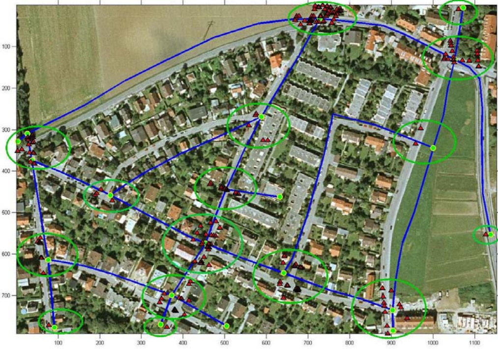
Fig. 5-9 Super junctions in green within the circular region and their estimated intersections in red in test area 1
