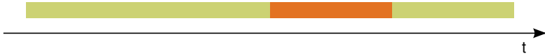
Figure 8.10: Schema of the reports inserted after the Shawn simulation for the defect scenario. The horizontal axis indicates the progressing simulation time. The green areas represent correct messages; the sending vehicle is working well. The red area in the middle marks a period, in which the vehicle is defect and, thus, disseminates wrong messages.
