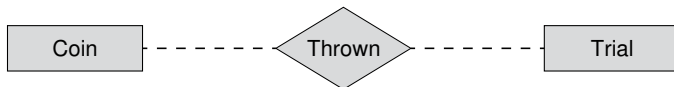
Figure 5.1: Graphical description of the entities and their relations in the coin toss example. The rectangles are entities; the diamond is a relationship.
