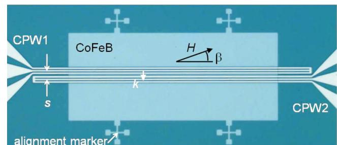
FIG. 1. Microscopy image of a CoFeB mesa with two integrated coplanar waveguides (CPWs). The center-to-center separation  $s$  of the two CPWs is 12  $\mu\text{m}$ . Orientations of in-plane magnetic field  $H$  and wave vector  $k$  are sketched.
