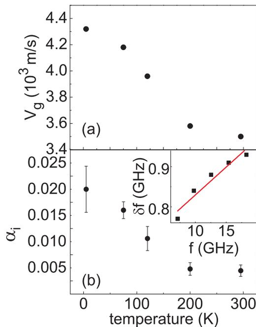
FIG. 5. (a) Group velocity measured on CoFeB in a perpendicular field of 1.9 T at different temperatures  $T$ . The eigenfrequency varies from 5.6 GHz to 7.2 GHz when  $T$  increases from 5 to 295 K. (b) Temperature dependence of intrinsic damping parameter  $\alpha_i$ . The inset shows  $\delta f$  vs  $f(H)$  at 295 K. The line reflects Eq. (2) leading to  $\alpha_i = 0.007$ .
