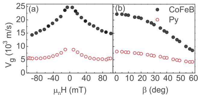
FIG. 3. (a) Group velocities of DE modes at room temperature as a function of applied field. Filled (open) circles denote CoFeB (permalloy). (b) Spin wave group velocity as a function of angle  $\beta$  when the in-plane field amounts to  $\mu_0 H = 20$  mT.
