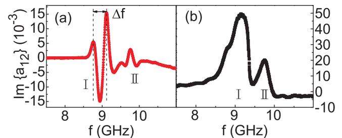
FIG. 4. (a) Imaginary part of the transmission signal obtained on CoFeB when the applied field of 1.9 T is perpendicular to the film plane.  $\Delta f$  indicates the phase shift of  $2\pi$  acquired by the MSFVWs. (b) Imaginary part of the reflection signal with an applied field of 1.9 T being perpendicular to the film plane. Both spectra were measured at 5 K.
