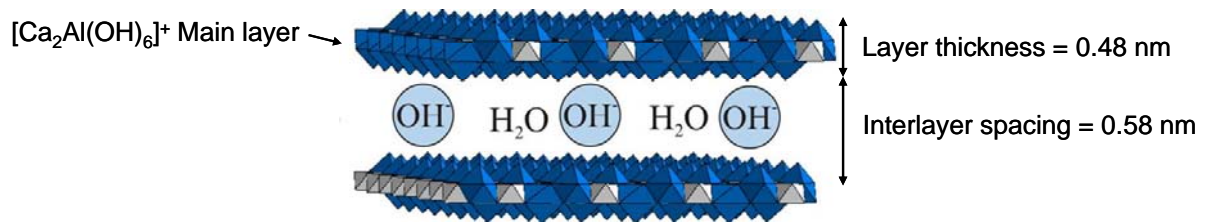
Fig. 1. Schematic illustration of the layer structure present in \text{C}_2\text{AH}_8 , a hydrocalumite mineral
