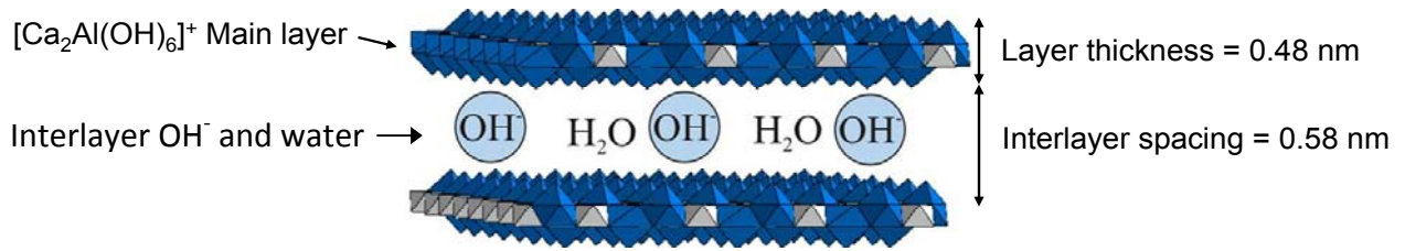
Figure 7. Schematic illustration of the layered structure of C_2AH_8
