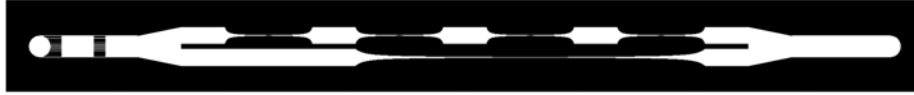
Figure 5.17: Lithography mask showing the geometry of the microfluidic rectangular "4xS vs. L" - setup. The device fulfills the condition given in eq. 5.19, which results in a Newtonian flowrate ratio X_N = 1 . As the extensional resistance of the channels is negligible as long as the Trouton ratio is small, a deviation from X_N can be directly associated with a high non-Newtonian extensional viscosity.
