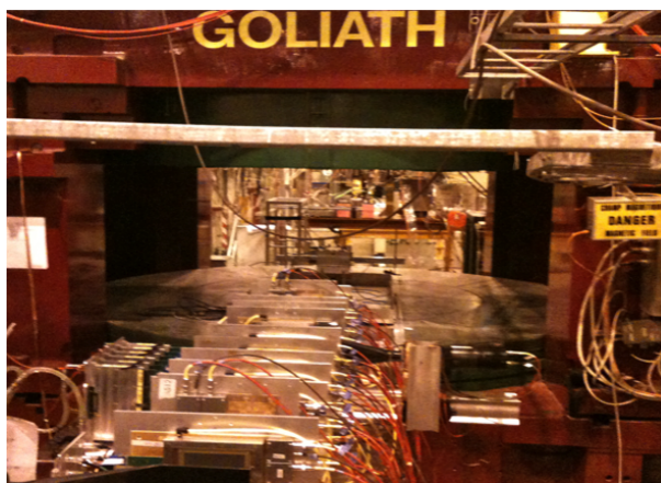
Figure 8.12: The 12 detectors on the test bench at the H4 beam line of the SPS in front of the GOLIATH magnet.
