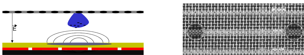
Figure 2.7: [Left] Principle of a simple resistive Micromegas. A resistive layer (in yellow) is deposited on the readout electrode. When a discharge (electron cloud in blue) starts from the micro-mesh, the resistive layer charges and creates an electric field that quenches the discharge. [Right] Photography of a detail of an active area of a resistive bulk Micromegas. Two pillars, in transparent coverlay, hold the metallic micro-mesh. Underneath the mesh, dark zones are resistive pads connected on top of copper strips at a pitch of 400\ \mu\text{m} .
