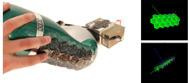
Fig. 1. 3D Reconstruction of a skin patch placed on a KUKA LWR arm
