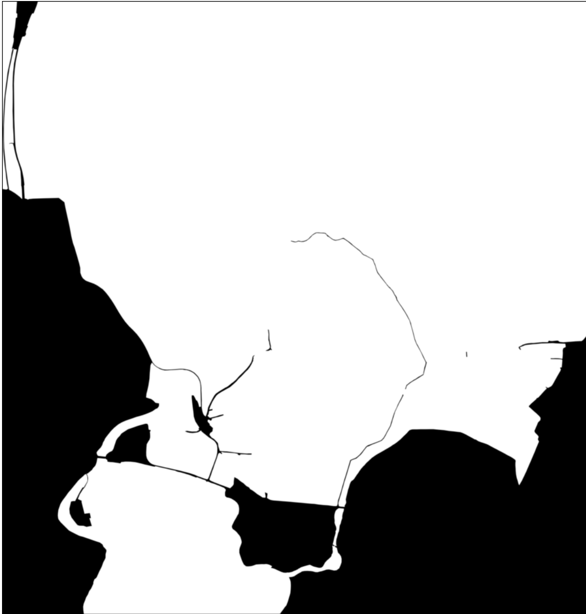
Figure 38. The generated reference data of the Elbe scenario with the aid of expert knowledge and the IKONOS image. (white: flooded areas, black: not flooded areas)
