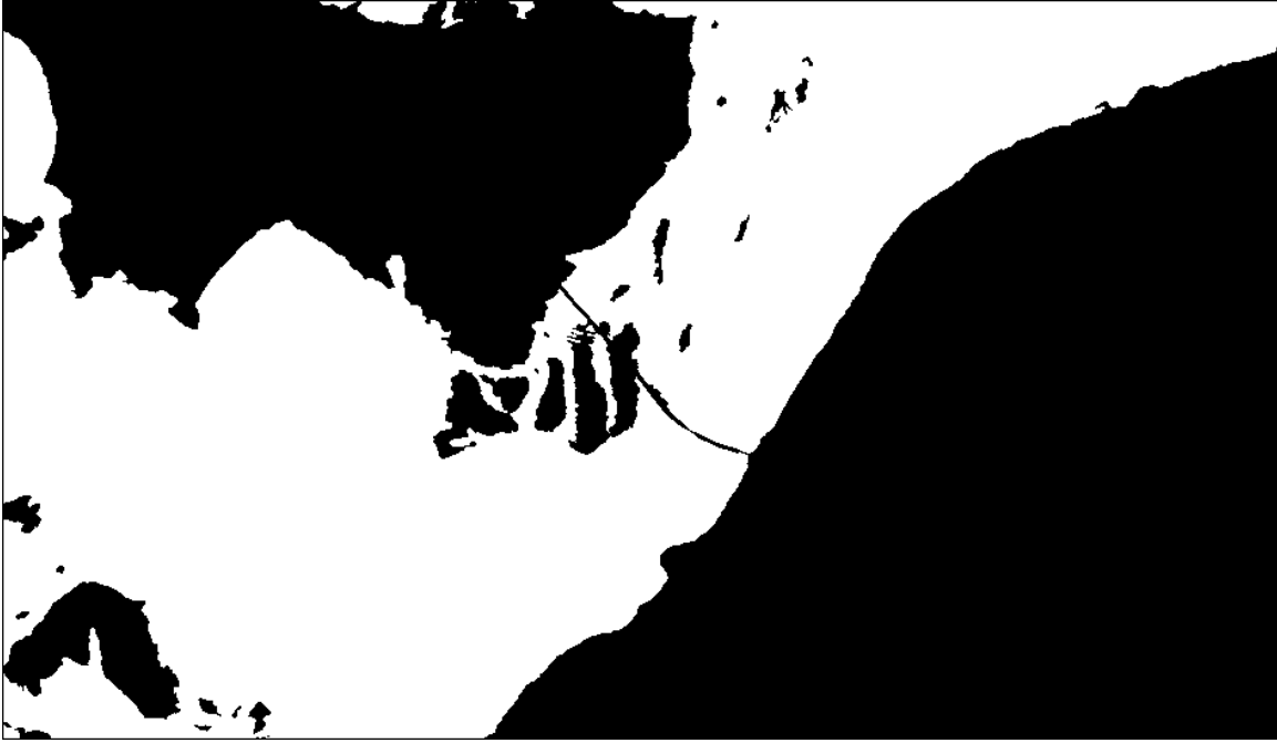
Figure 39. The generated reference data for the RapidEye image of the Chobe scenario with the aid of the image data. (white: flooded areas, black: not flooded areas)
