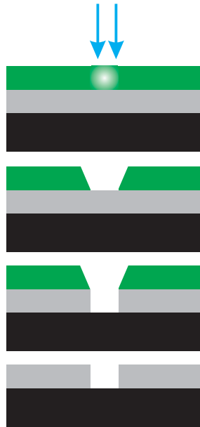
Figure 3.2: Optical lithography process is schematically shown. A substrate (black, e.g. Si) comprising an additional layer (gray, e.g. \text{SiO}_2 ) is covered by a photoresist (green, e.g. positive resist). By illuminating the photoresist through a mask, certain areas of the resist are exposed, and chemically changed. In the case of a positive resist, the exposed areas become soluble in a developer (usually a base). This creates a window in the resist and further structuring of the surface can be done, like chemically etching of the additional layer. After removing the remaining resist in e.g. acetone, a microscale structured surface is obtained.
