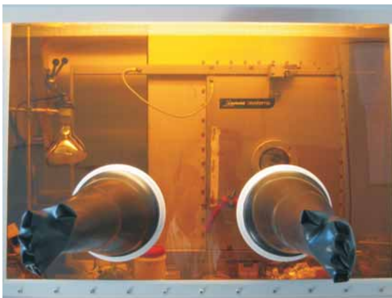
Figure 3.1: Photograph of UNIVEX 350G: The thermal evaporator is located inside a glovebox in order to guarantee a nitrogen atmosphere. Oxidation of metals or degradation of polymers is slowed.
