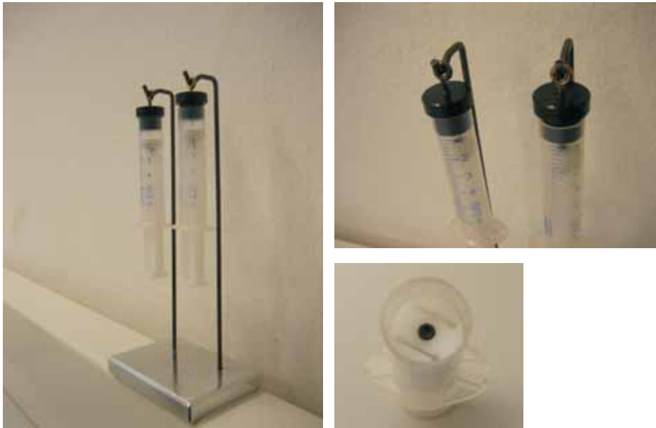
Figure A.1: Photograph of MBE stamp holder for SAM formation
