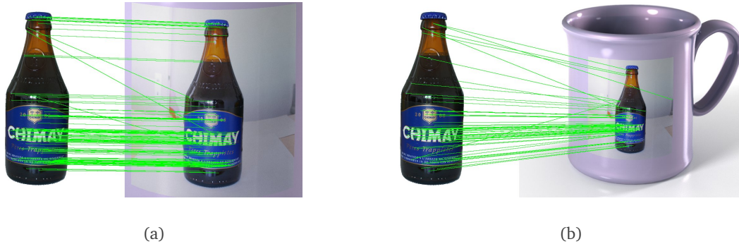
Figure 1.1: (a) A good match between a template image representing the object of interest (left) and a scene (right). (b) However, it turns out, that the beer bottle is a sticker put on the surface of a mug (image courtesy of Radu Bogdan Rusu [16]).
