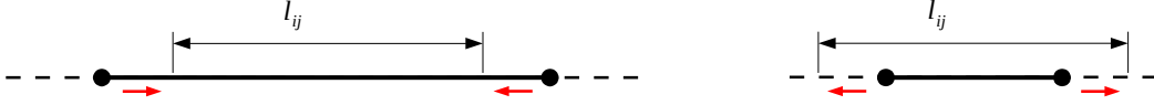
Figure 4.5: The vertices of a stretched (compressed) edge are translated innwards (outwards) until the edge attains its rest length l_{ij} .
