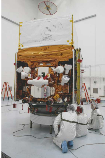
Figure 1.3 The Fermi Gamma-Ray Space Telescope being prepared for launch vehicle integration at Cape Canaveral. On top is the LAT with its reflective covering. Six of the GBM NaI detectors and one BGO detector can be seen on the side of the spacecraft. Photo credit: NASA/Kim Shiflett. Picture and caption taken from Meegan et al. (2009).
