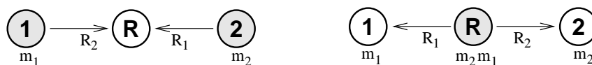
Figure 3. Bidirectional relaying in a three-node network, where nodes 1 and 2 exchange their messages m_1 and m_2 with the help of the relay node using a decode-and-forward protocol.
