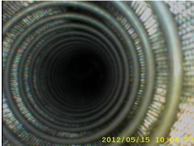
Figure 3.14: Spiral spring to keep the sVCHP mesh in place
