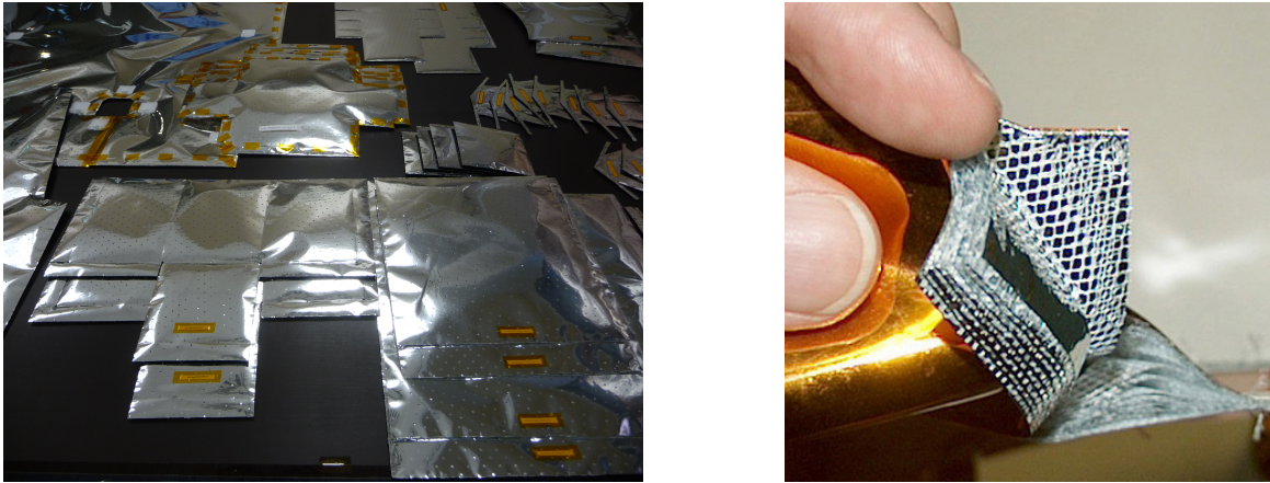
Figure 5.2: Multi-layer insulation lay-up (left: eROSITA MLI blankets; right: image credit to AerospaceEd.org)
