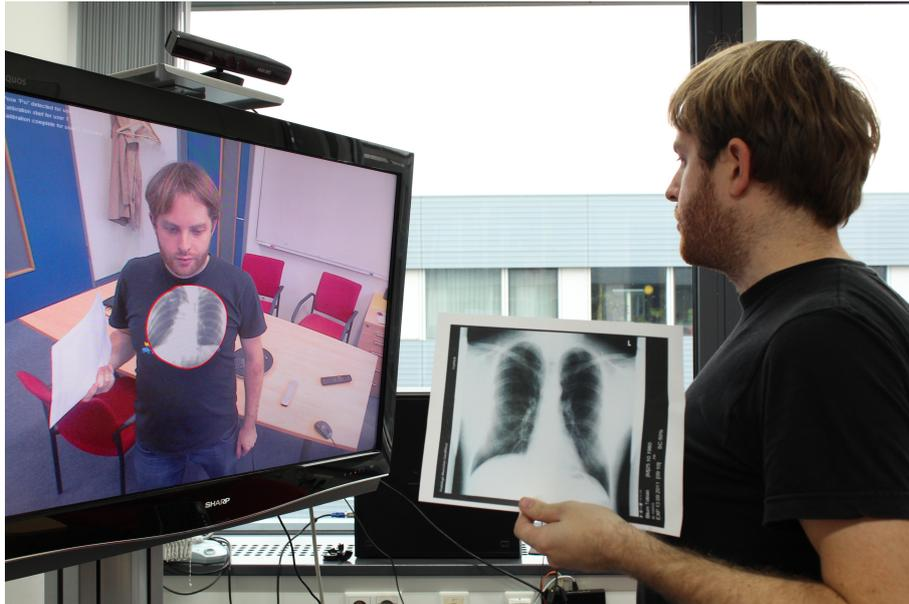
Figure 5.4.: The magic mirror shows a simulated X-ray (DRR). For comparison, the image printed on the sheet of paper shows a real X-ray of the same person.
