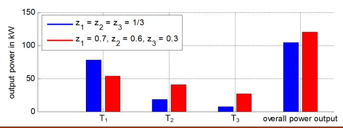
Considering the interaction within a Wind Farm is needed for control to increase the overall power output.
