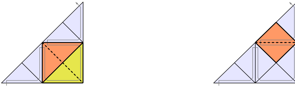
Figure 3.13: Incorrect coarsening – merging non-siblings leads to erroneous triangle position (left) or to a square (right).
